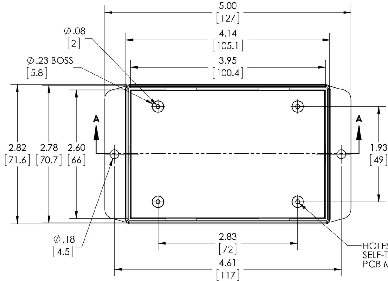
HOLES ACCEPT M2.6 x 6mm LG. SELF-TAPPING SCREWS FOR PCB MOUNTING
