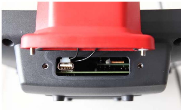
Figure 5.11: Service USB under the antenna cap
