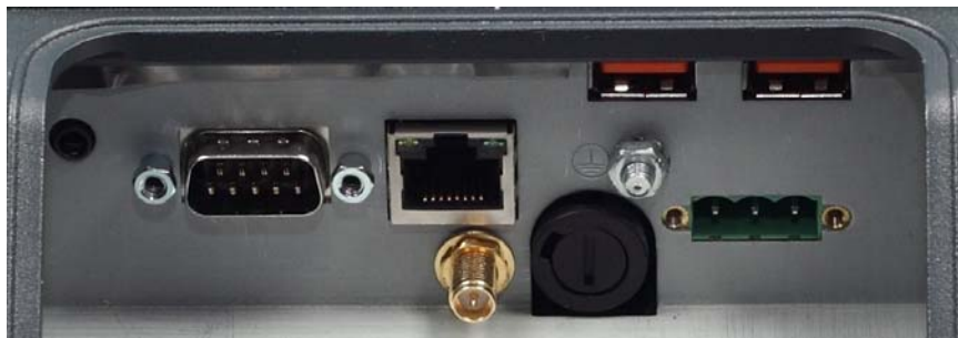
Figure 5.7: External connectors with optional ext. antenna
