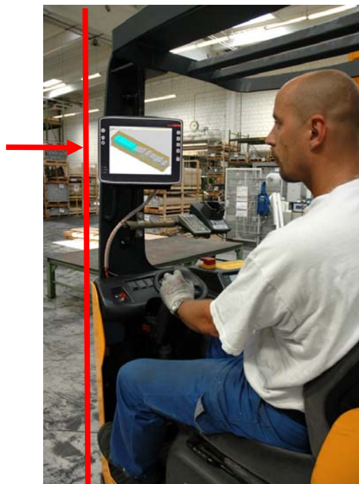
Figure 7.2: Position of the MTC 6 on a forklift
