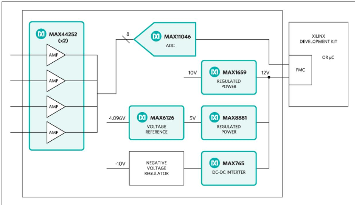
Figure 1. The Petaluma subsystem design block diagram.
