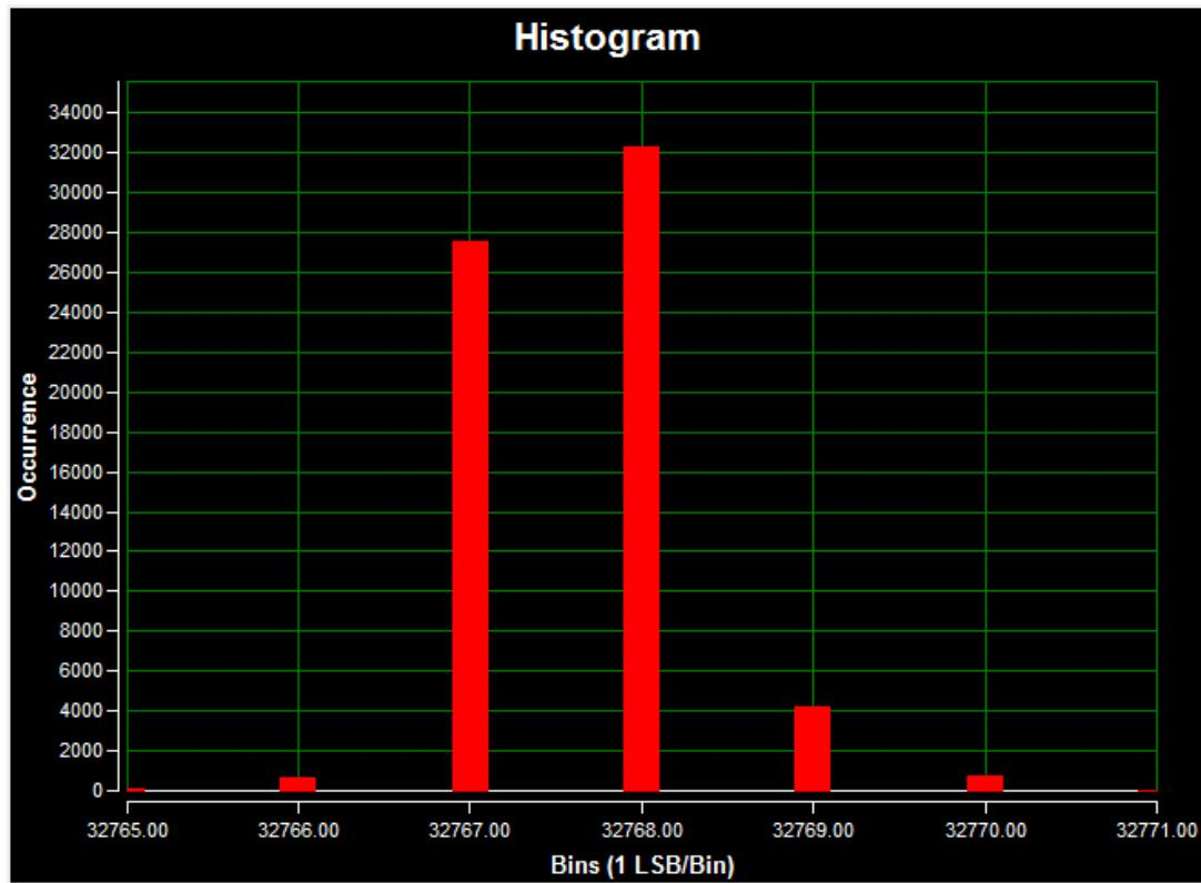
Figure 6. DC histogram for channel 7 (AIN7) using on-board power; a 0V DC input signal; a 250ksps sample rate; 65536 samples; a code spread of 21 LSBs with 97.7% of the codes falling within the three center LSBs; and a standard deviation of 0.711 at room temperature.
