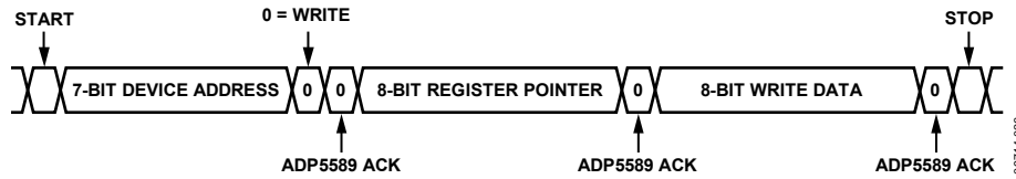
Figure 27. I 2 C Single-Byte Write Sequence
