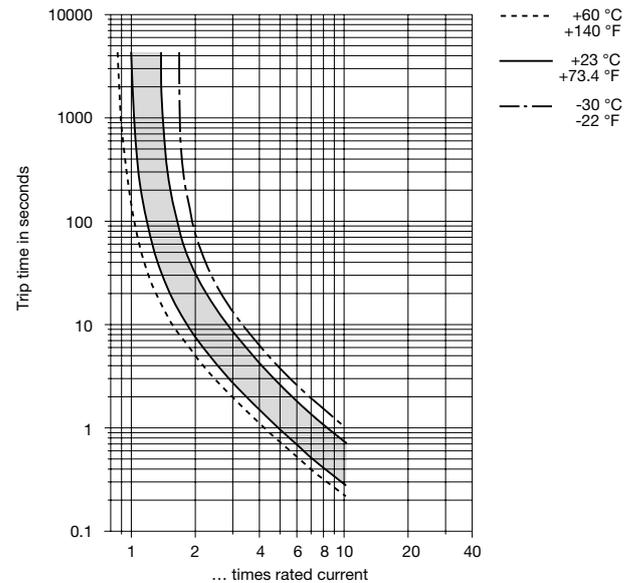
The time/current characteristic depends on the ambient temperature. In order to eliminate nuisance tripping, please multiply the current rating by a derating factor (see chapter Technical Information)
