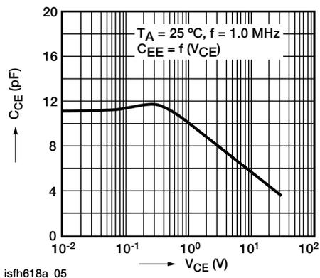
Fig. 8 - Transistor Capacitance
