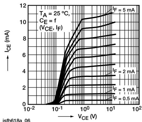
Fig. 9 - Output Characteristics
