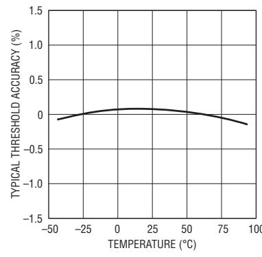
**Figure 5. Typical Threshold Accuracy vs Temperature**
