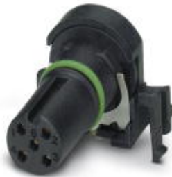
Sensor/actuator flush-type connector, socket, 5-pos., A-coded, shielded, with angled solder connection, only contact insert
