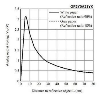
**Note:** Because of some basic trigonometry within the triangle from the emitter to reflection spot to receiver, the output of the detector is non-linear with respect to the distance being measured.
