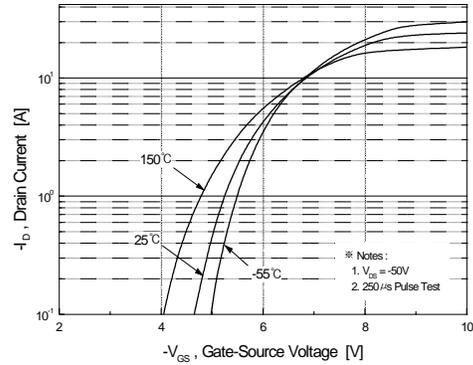
Figure 2. Transfer Characteristics
