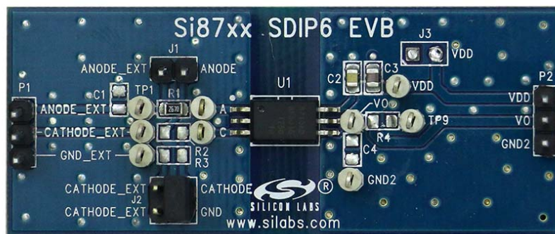
Figure 3. Si871x SDIP6 Evaluation Board Overview
