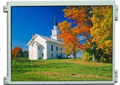
Kyocera's 12.1-inch diagonal SVGA resolution TFT LCD provides the ideal solution for industrial applications. It features a wide viewing angle measuring +/- 80° for both vertical and horizontal (at CR>10). It offers a backlight lifetime of 70K hours, a luminance of 500cd/m<sup>2</sup> and a 1000:1 contrast ratio, with standard LVDS interface and wide operating temperature range. Plus the constant current circuit (CCC) is built-in to simplify the design.
