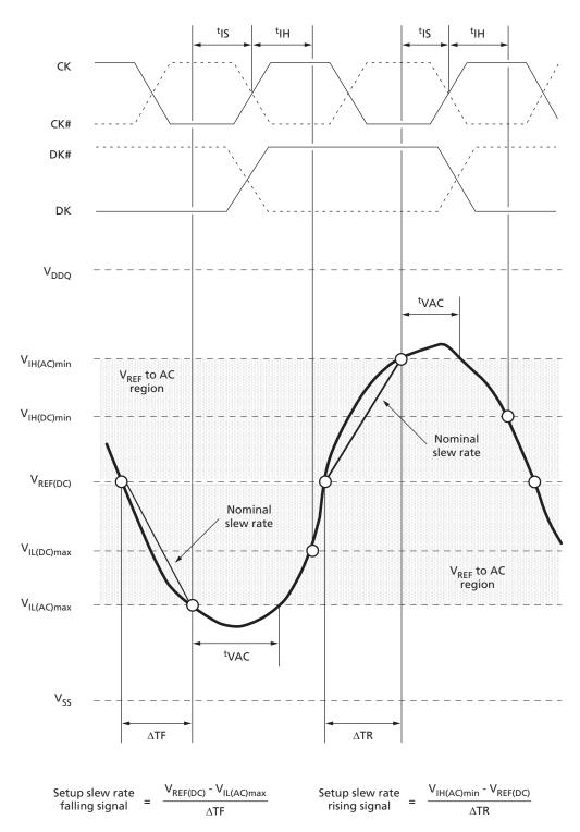
Note: 1. Both the clock and the data strobe are drawn on different time scales.
