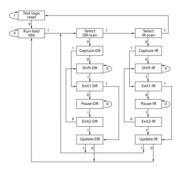
**Figure 69: TAP Controller Functional Block Diagram**
