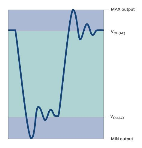
**Figure 17: Differential Output Signal**
