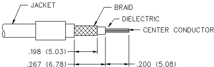
1. Identify connector parts. (2 piece parts)
