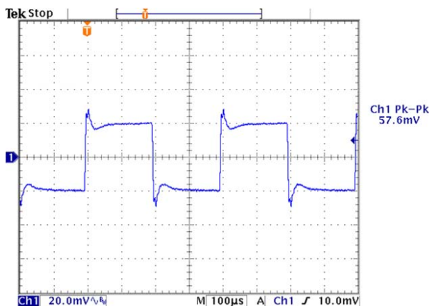
Figure 21. Transient Response with Optimal Voltage Positioning
