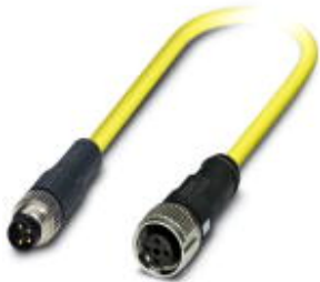
Sensor/Actuator cable, 4-position, PVC, Yellow RAL 1021, Plug straight M8, on Socket straight M12-SPEEDCON, A-coded, Cable length: 1.5 m
