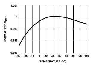
FIGURE 1. REFERENCE VOLTAGE vs TEMPERATURE
