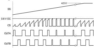
FIGURE 7. PULSE-BY-PULSE OC BEHAVIOR DURING SS
