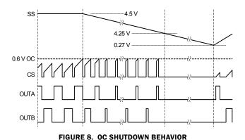
Figure 8 portrays the typical delayed overcurrent shutdown behavior. Once SS has discharged to 4.25V, the outputs are disabled and remain that way until SS has discharged to 0.27V, and then a new SS cycle begins.
