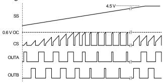
FIGURE 7. PULSE-BY-PULSE OC BEHAVIOR DURING SS
