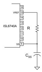
FIGURE 10. MODIFYING OC SHUTDOWN TIMING
