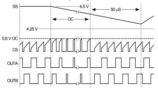
FIGURE 9. OC RECOVERY PRIOR TO SHUTDOWN
