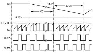
FIGURE 9. OC RECOVERY PRIOR TO SHUTDOWN
