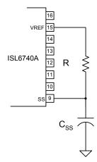
FIGURE 10. MODIFYING OC SHUTDOWN TIMING
