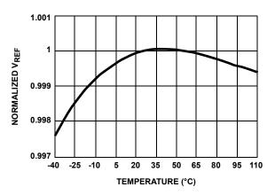
FIGURE 1. REFERENCE VOLTAGE vs TEMPERATURE
