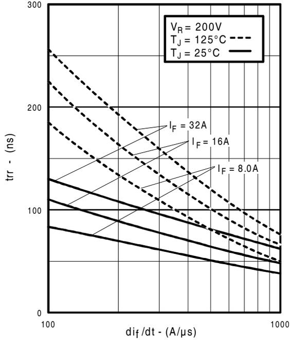
Fig. 14 - Typical Reverse Recovery vs.  $di/dt$
