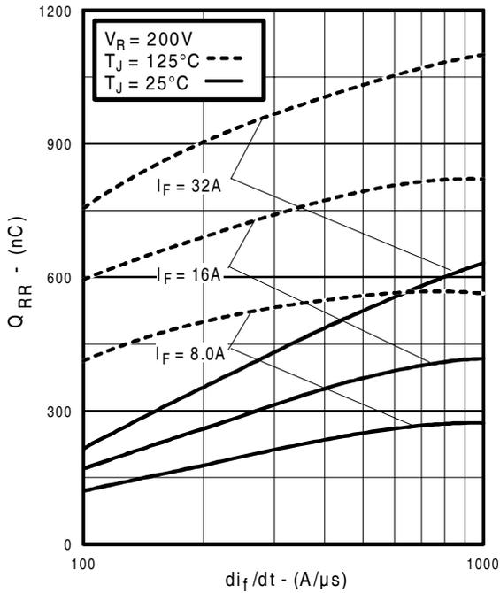
Fig. 16 - Typical Stored Charge vs.  $di/dt$
