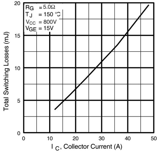
**Fig. 11** - Typical Switching Losses vs. Collector Current
