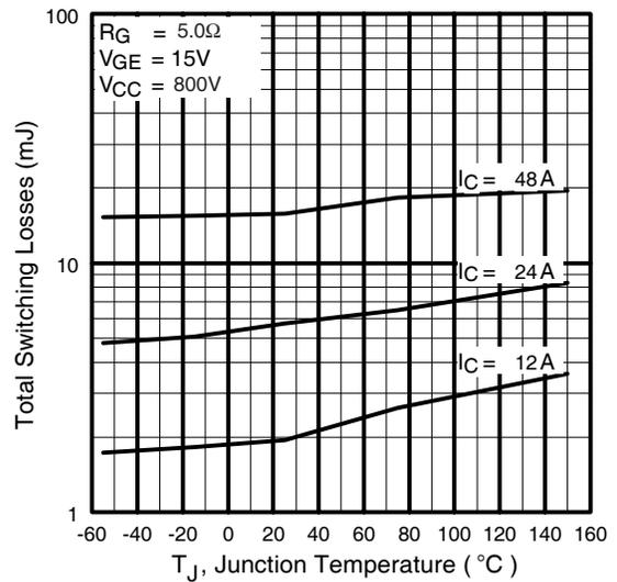
**Fig. 10** - Typical Switching Losses vs. Junction Temperature
