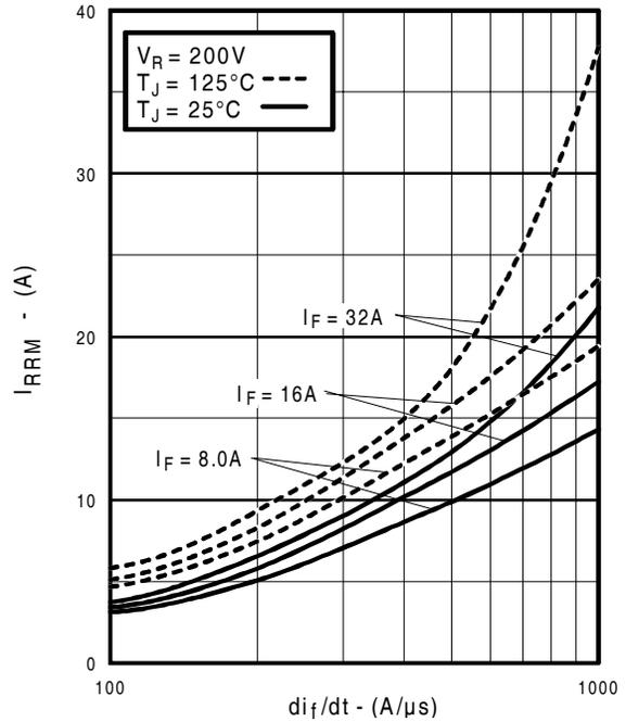
Fig. 15 - Typical Recovery Current vs.  $di/dt$
