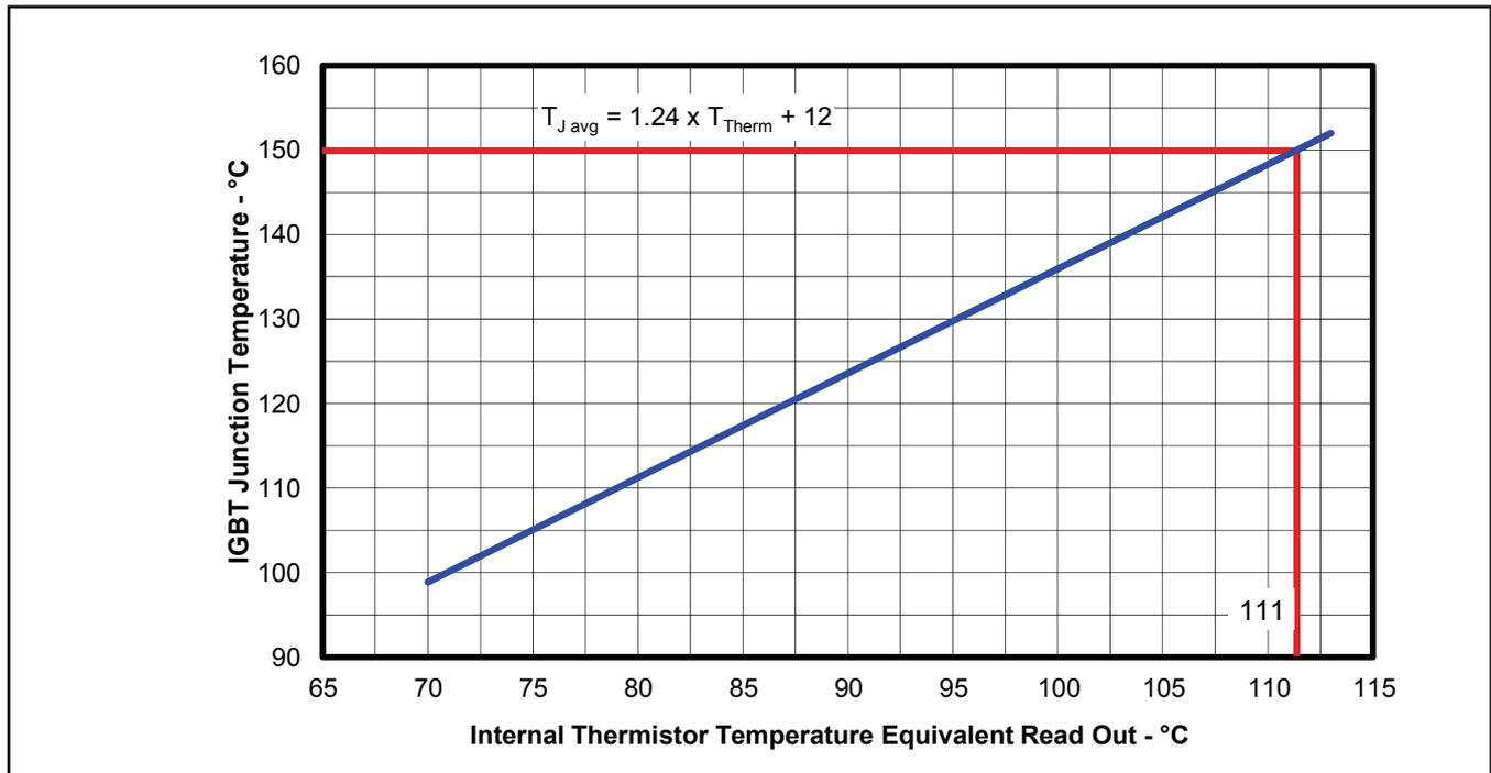
**Figure 16** Typical Tj vs Tth correlation, sinusoidal modulation, V<sub>DC</sub>=300V, I<sub>phase</sub>=5Arms, f<sub>sw</sub>=16kHz, f<sub>mod</sub>=50Hz, MI=0.8, PF=0.6
