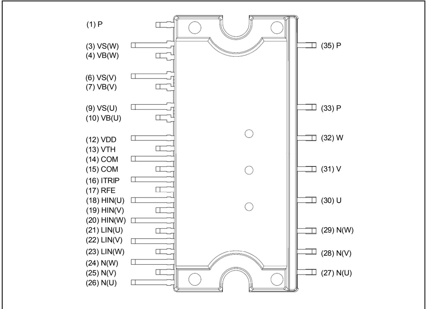
Figure 2 Pin configuration
