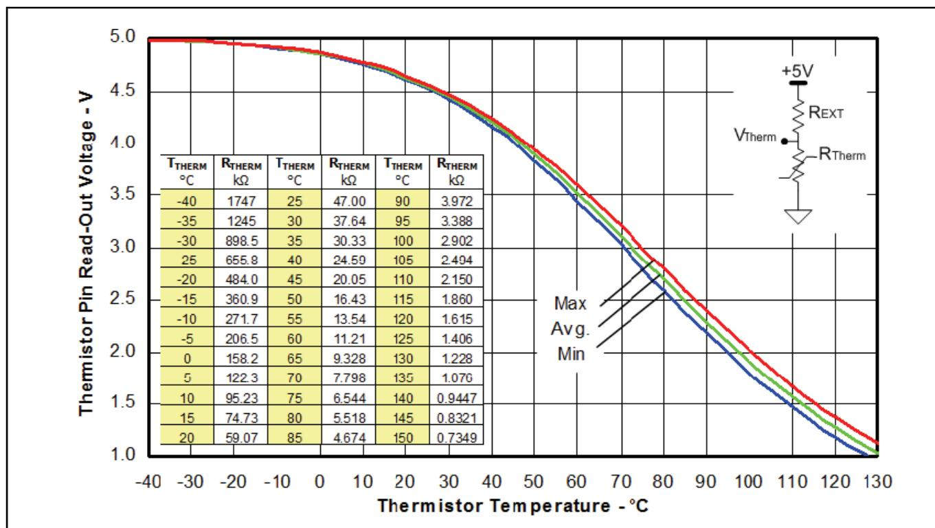
**Figure 7** Thermistor readout vs. temperature (with 4.7kohm R<sub>EXT</sub> pull-down resistor) and typical thermistor resistance values vs. temperature table
