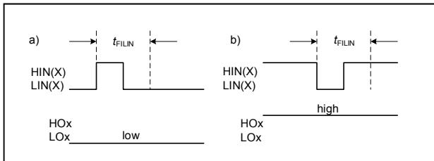
**Figure 4** Input filter timing diagram
