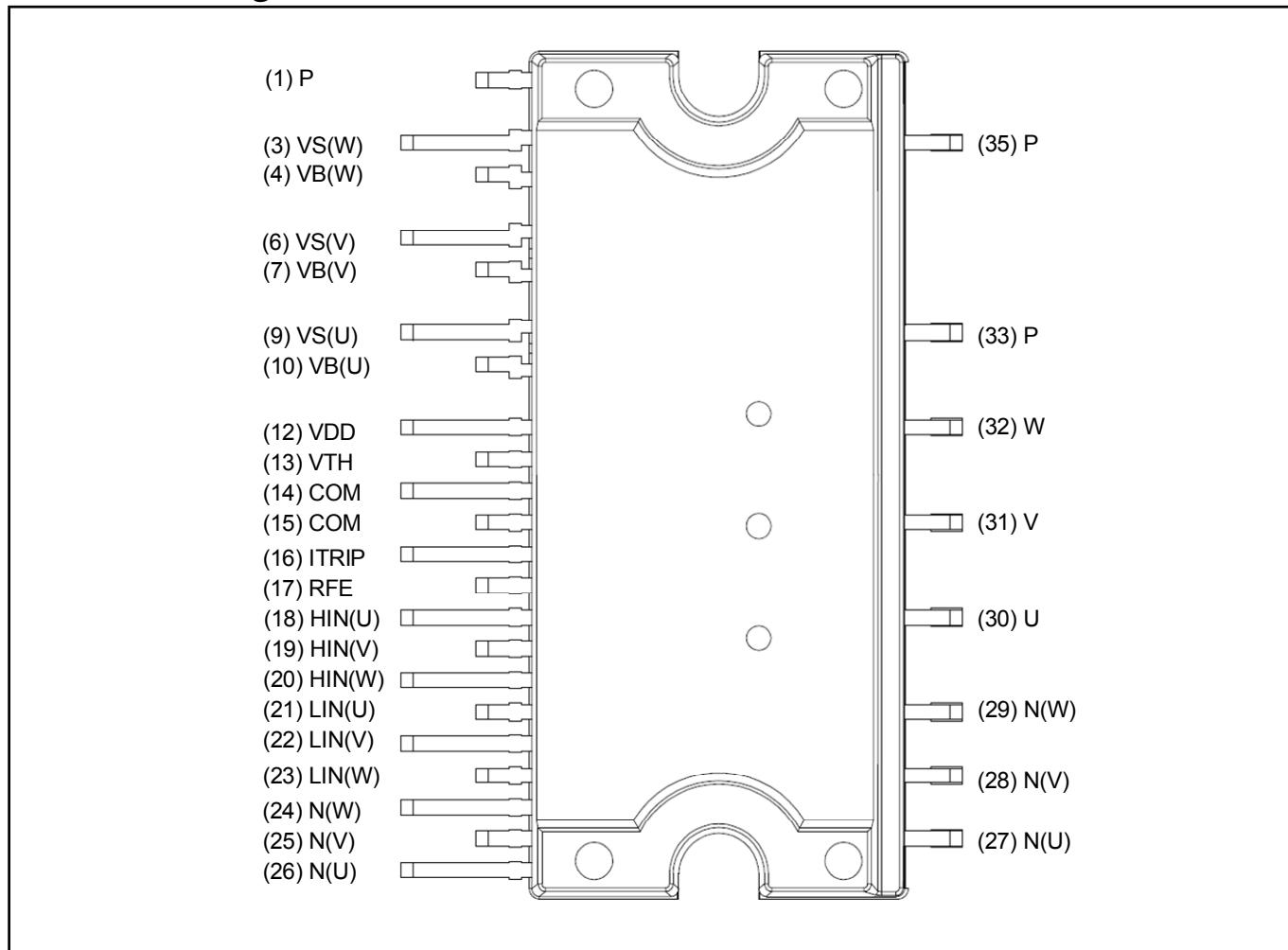
**Figure 2** Pin configuration
