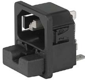
IEC connector C14 with fuse holder 2-pole Snap-in mounting from front side Solder or quick connect terminals Snap-in version
