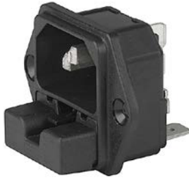
IEC connector C14 with fuse holder 2-pole Screw-on version from front or rear side Solder or quick connect terminals Screw-on mounting
