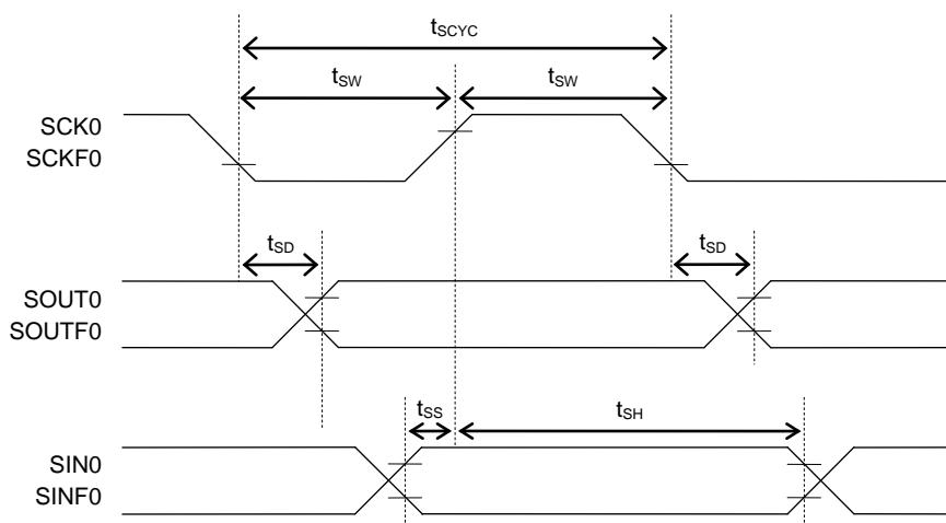
AC characteristics (I<sup>2</sup>C Bus interface : Standard mode 100kHz)(V<sub>DD</sub>=1.8 to 5.5V, V<sub>SS</sub>=0V, Ta=-40 to +85°C, unless otherwise specified)
