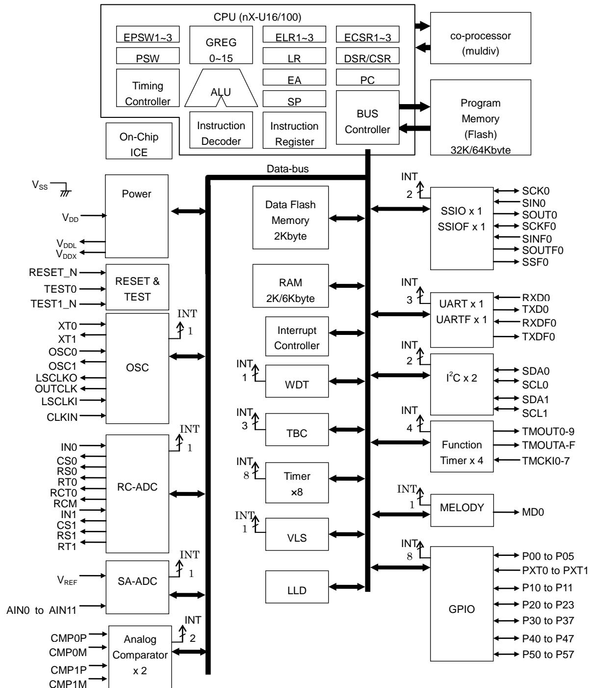
**Figure 1. Block Diagram of ML620Q503H/Q504H**
