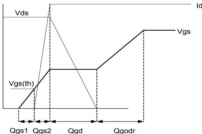
**Fig 13a.** Gate Charge Waveform
