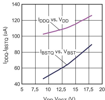
**TYPICAL PERFORMANCE CHARACTERISTICS (continued)** $V_{DD} = 12V$ ,  $V_{SS} = V_{SW} = 0V$ ,  $T_A = 25^\circ C$ , unless otherwise noted.
