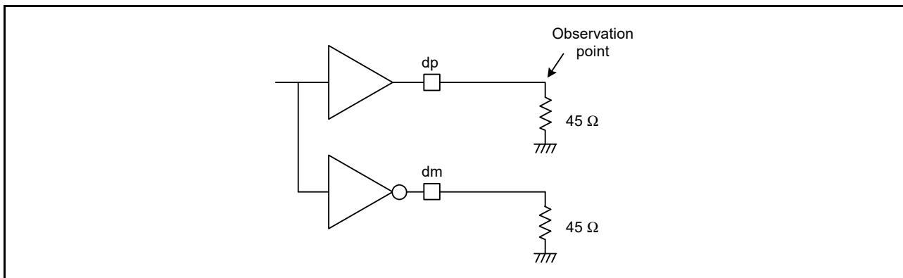
**Figure 5.82 Test Circuit (High-Speed)****Table 5.47 Battery Charge Characteristics (USBA only)**
