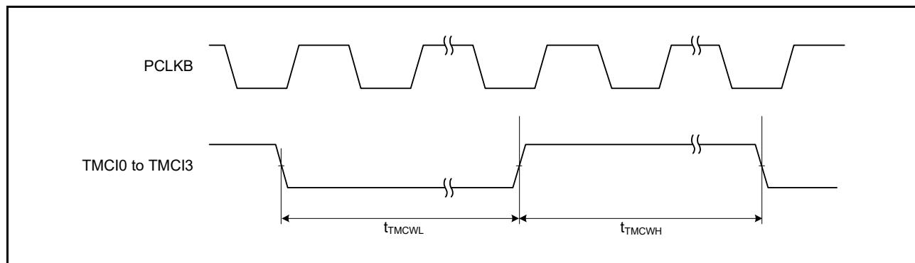
**Figure 5.36 TMR Clock Input Timing****Table 5.28 CMTW Timing**
