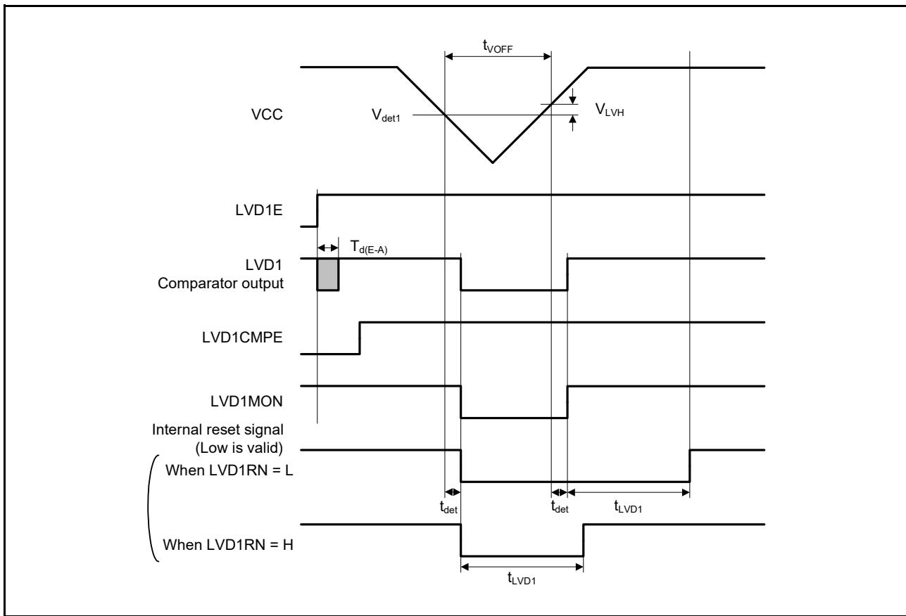
Figure 5.85 Voltage Detection Circuit Timing ( $V_{det1}$ )
