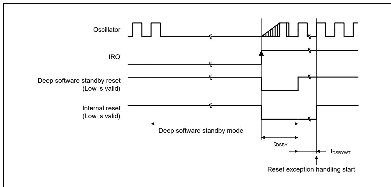
**Figure 5.13 Deep Software Standby Mode Cancellation Timing**
