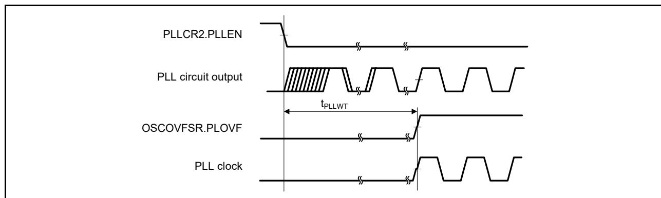
**Figure 5.10 PLL Clock Oscillation Start Timing****Table 5.19 Sub-Clock Timing**
