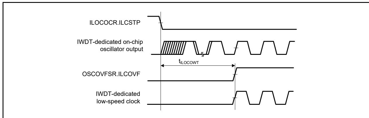
**Figure 5.7 IWDT-dedicated Low-Speed Clock Oscillation Start Timing**
