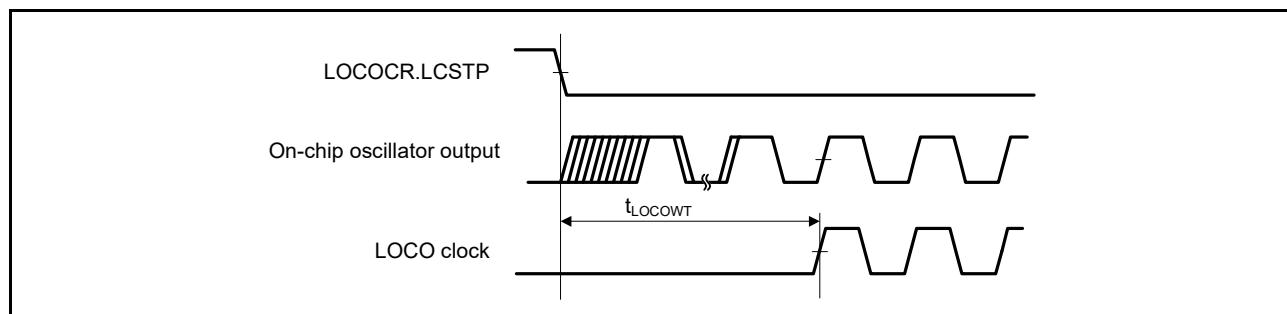
**Figure 5.6 LOCO Clock Oscillation Start Timing**
