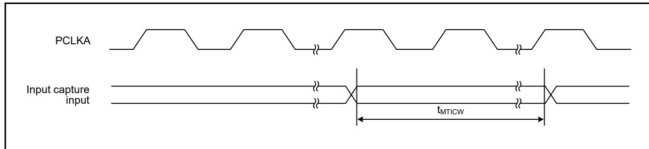
**Figure 5.38 MTU3 Input Capture Input Timing**
