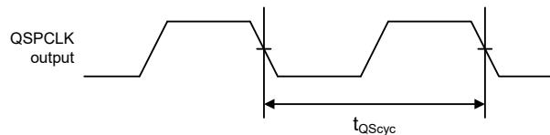
**Figure 5.53 QSPI Clock Timing**
