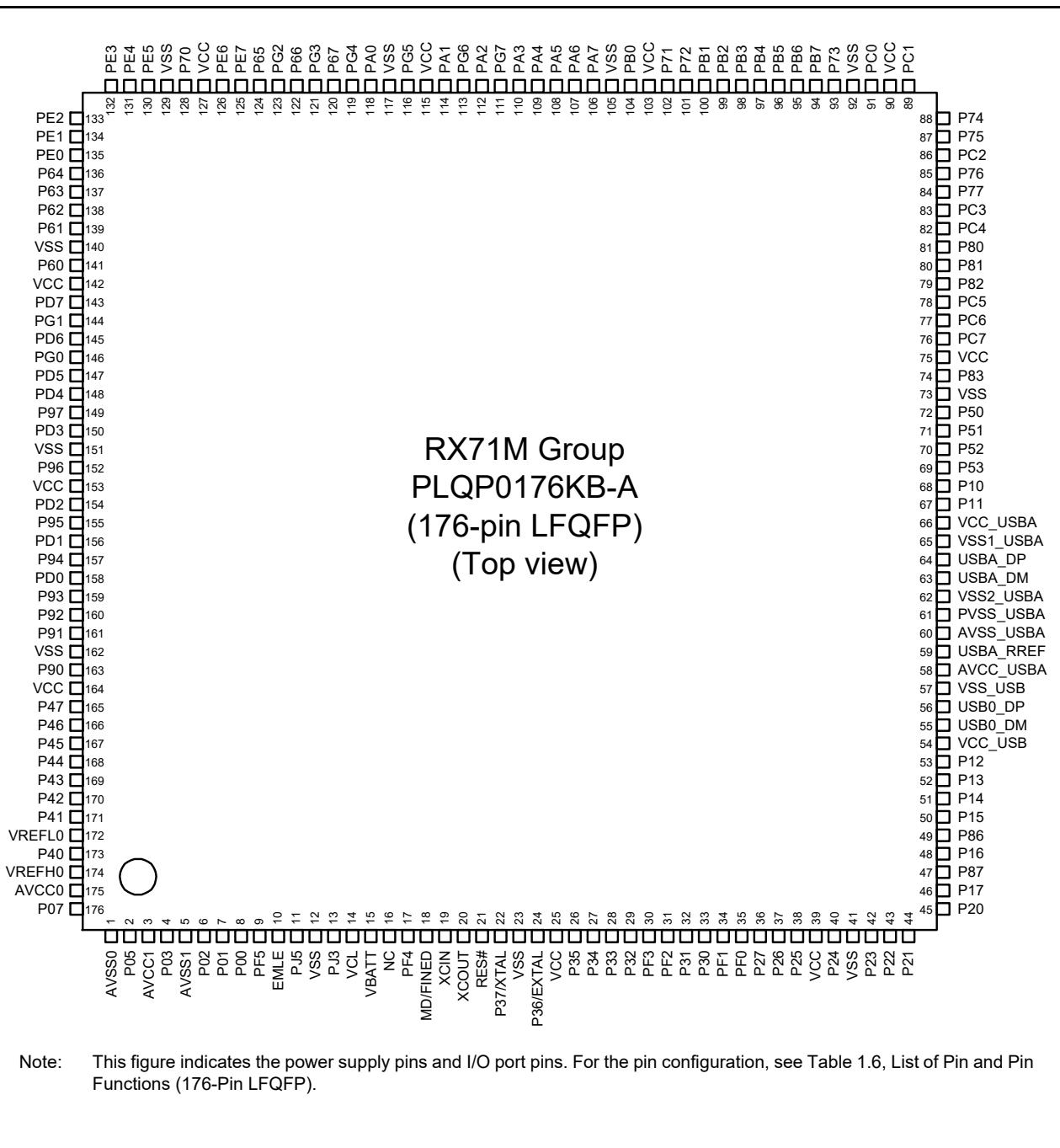
Note: This figure indicates the power supply pins and I/O port pins. For the pin configuration, see Table 1.6, List of Pin and Pin Functions (176-Pin LFQFP).
