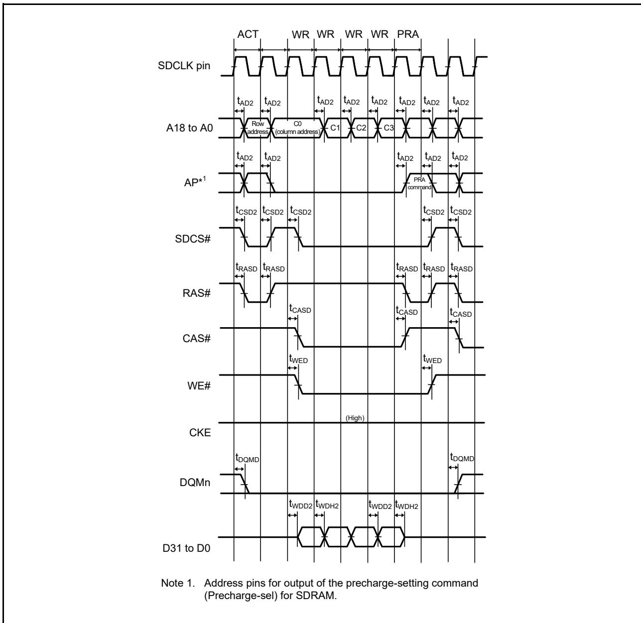
**Figure 5.26 SDRAM Space Multiple Write Bus Timing**
