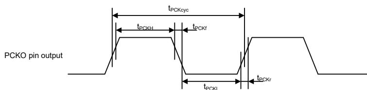
**Figure 5.73 PDC Output Clock Timing**
