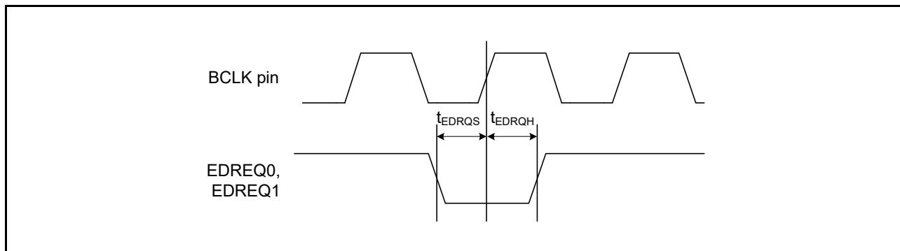
**Figure 5.30 EDREQ0 and EDREQ1 Input Timing**
