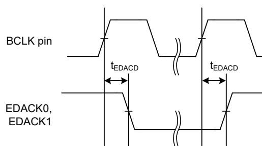
Figure 5.32 EDACK0 and EDACK1 Single-Address Transfer Timing (for SDRAM)
