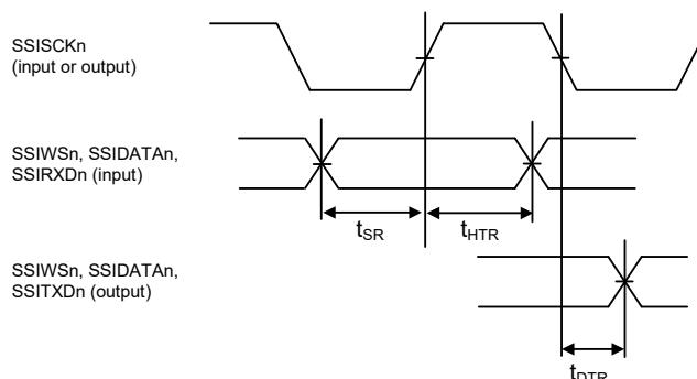
**Figure 5.58 Transmit/Receive Timing (SSISCKn Rising Synchronous)**
