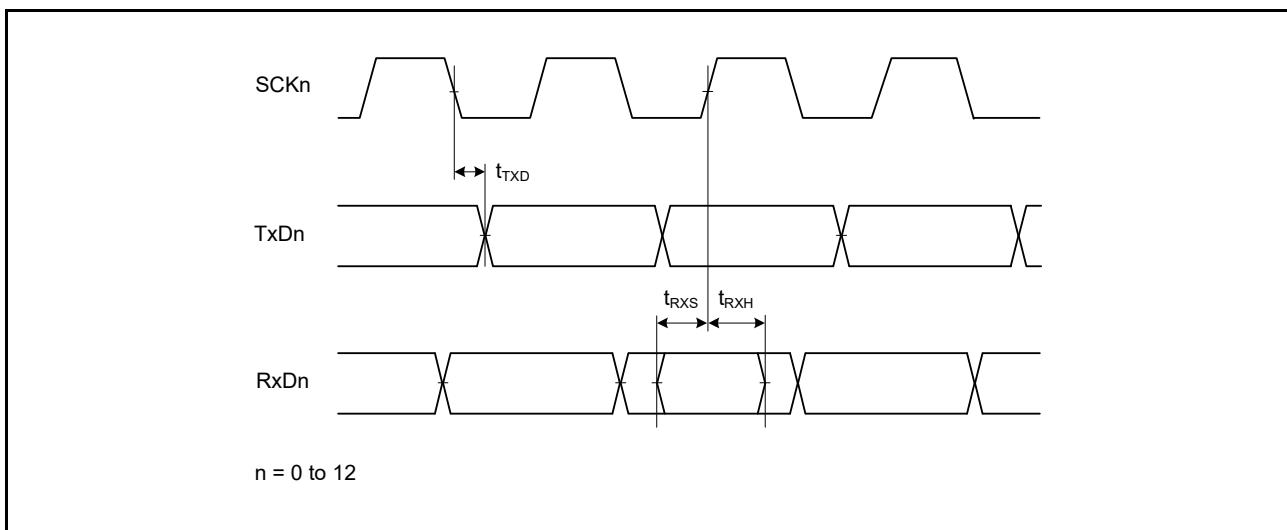
Figure 5.45 SCI Input/Output Timing: Clock Synchronous Mode
