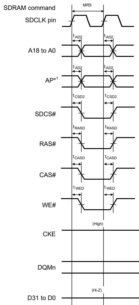
Note 1. Address pins for output of the precharge-setting command (Precharge-sel) for SDRAM.
