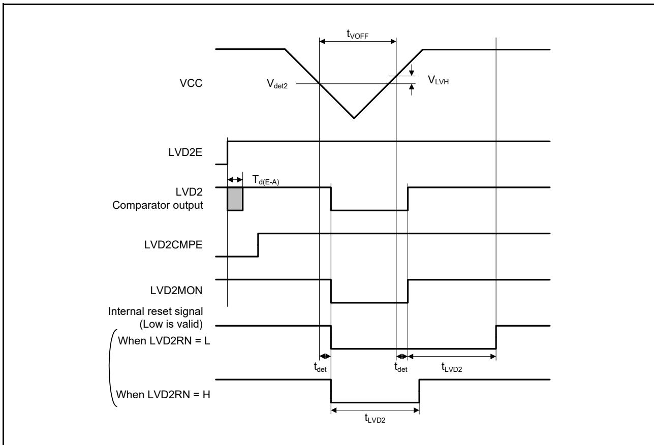
Figure 5.86 Voltage Detection Circuit Timing ( $V_{det2}$ )
