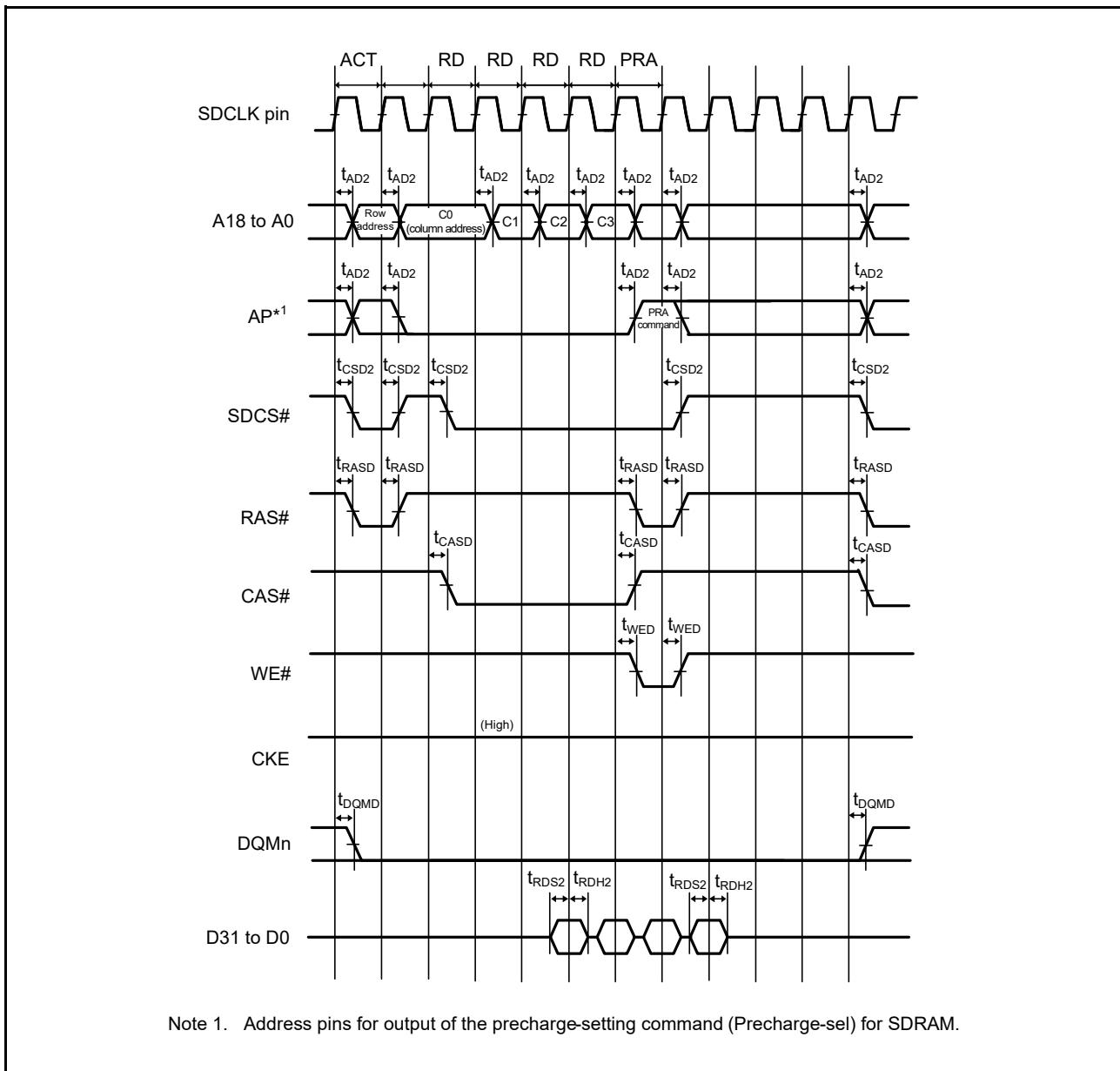
**Figure 5.25 SDRAM Space Multiple Read Bus Timing**
