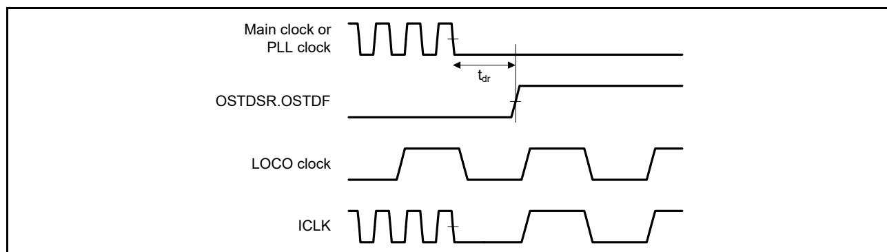
**Figure 5.87 Oscillation Stop Detection Timing**
