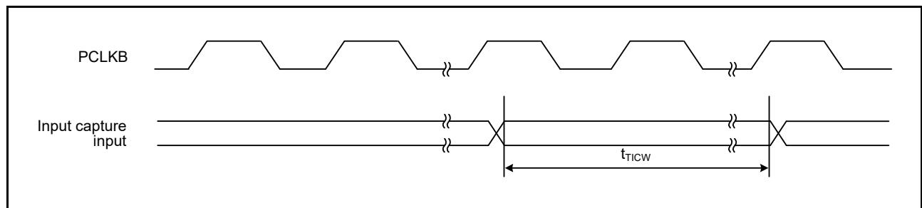
**Figure 5.34 TPU Input Capture Input Timing**
