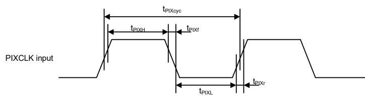
**Figure 5.72 PDC Input Clock Timing**
