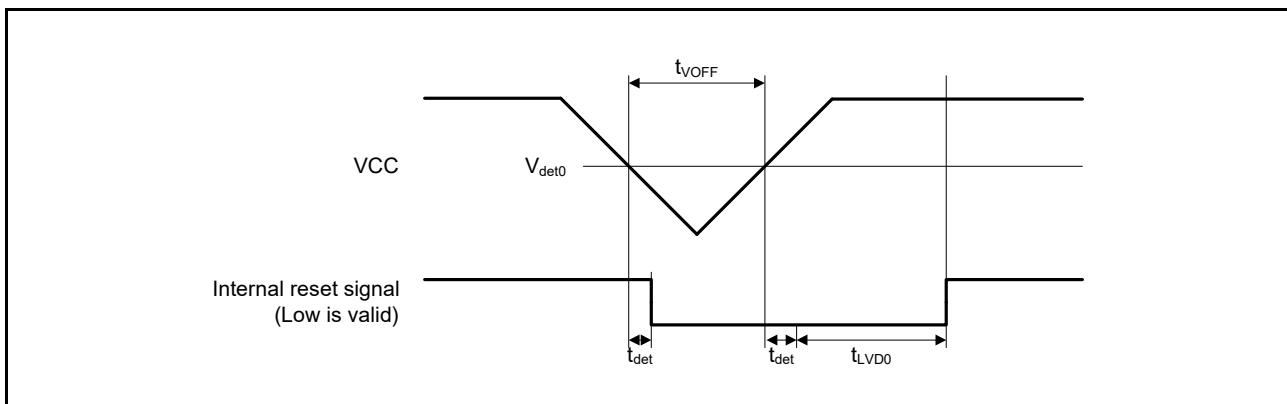
Figure 5.84 Voltage Detection Circuit Timing ( $V_{det0}$ )
