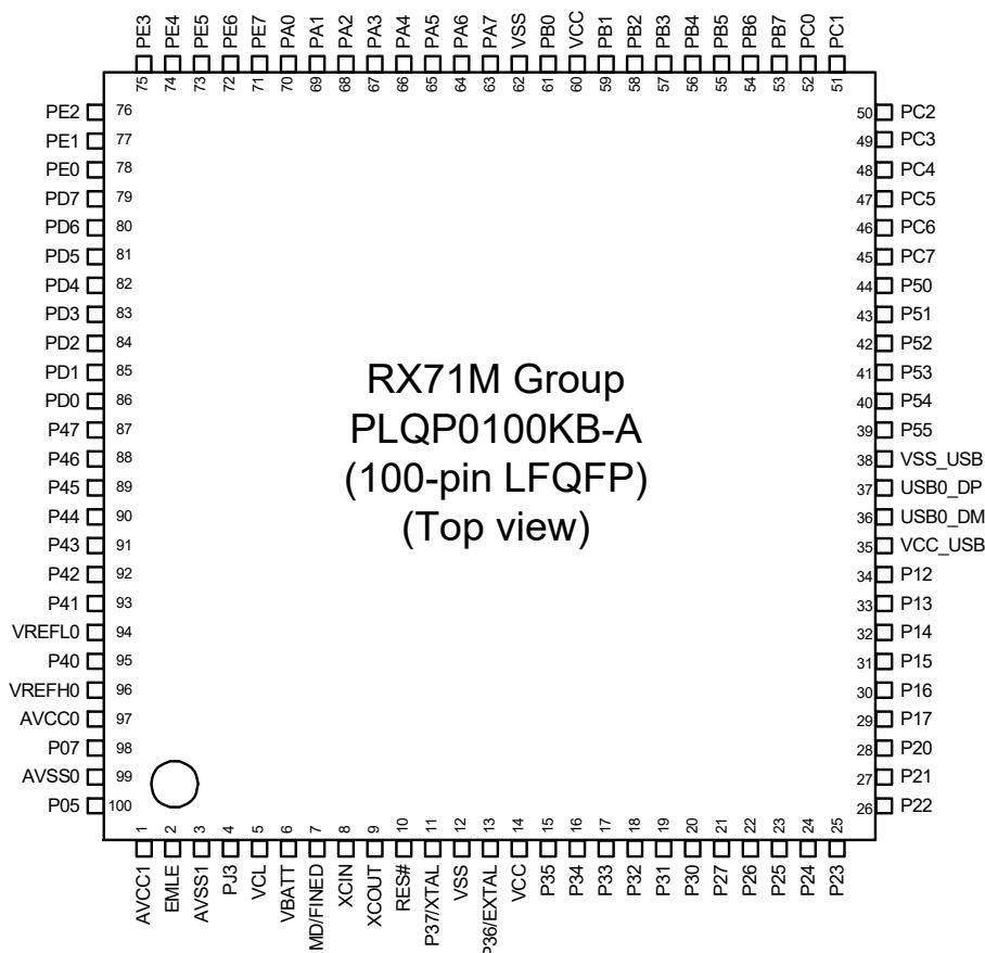
Note: This figure indicates the power supply pins and I/O port pins. For the pin configuration, see Table 1.10, List of Pin and Pin Functions (100-Pin LFQFP).
