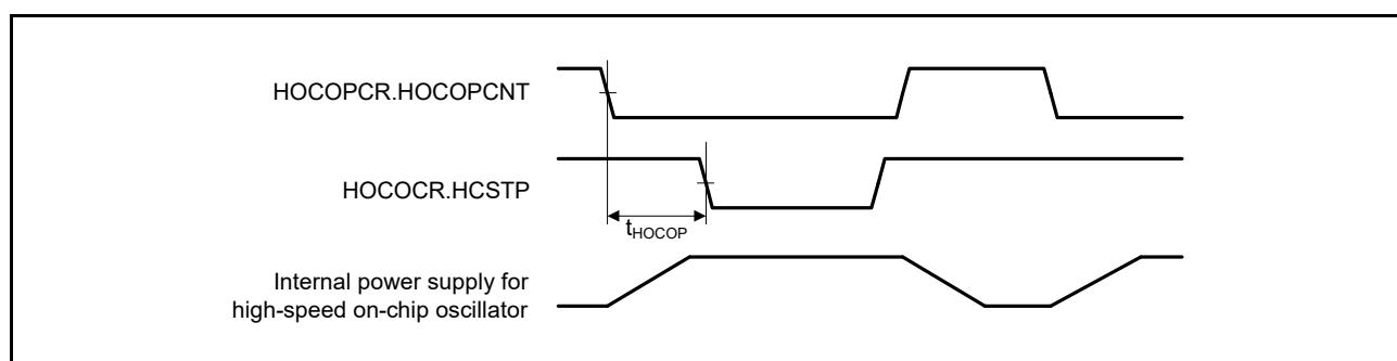
**Figure 5.9 High-Speed On-Chip Oscillator Power Supply Control Timing**
