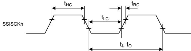
**Figure 5.57 Clock Input/Output Timing**
