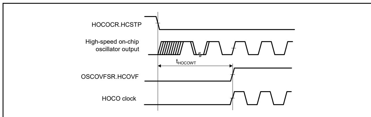
**Figure 5.8 HOCO Clock Oscillation Start Timing (Oscillation is Started by Setting the HOCOCR.HCSTP Bit)**
