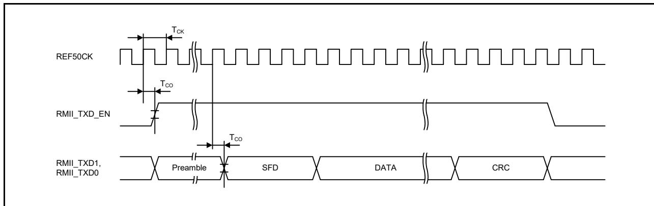
**Figure 5.63 RMII Transmission Timing**
