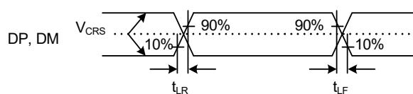
**Figure 5.75 DP and DM Output Timing (Low Speed)**
