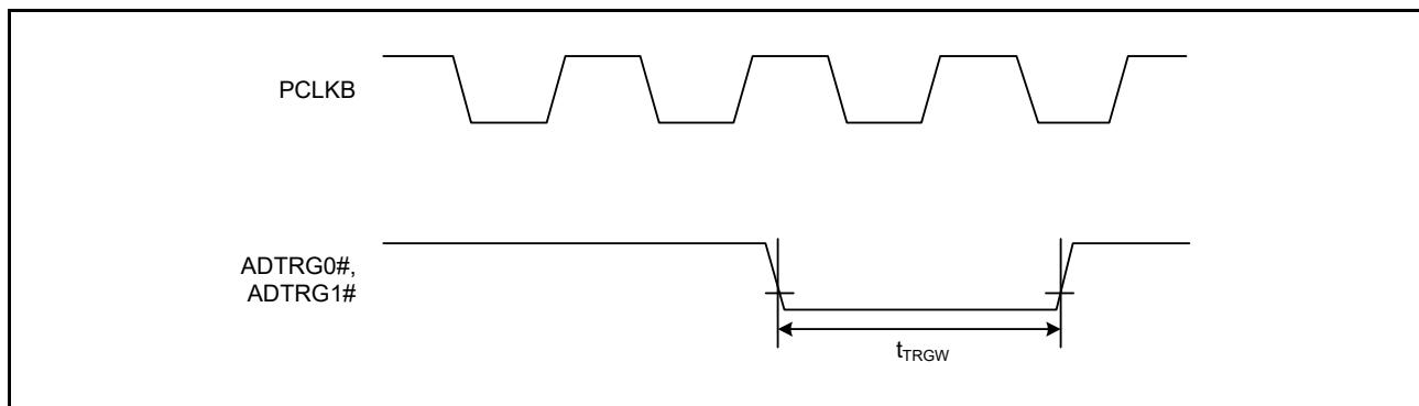
**Figure 5.43 A/D Converter Trigger Input Timing****Table 5.33 CAC Timing**
