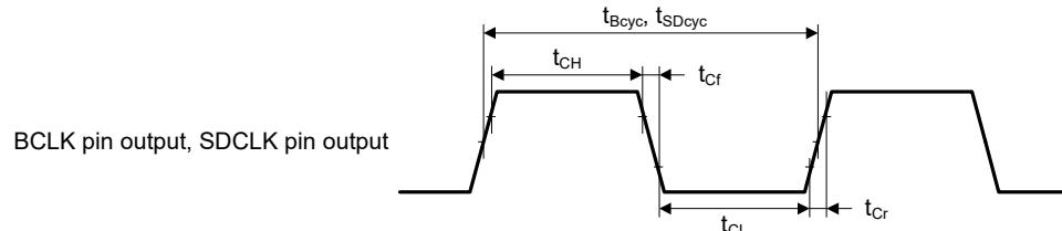
Test conditions: VOH = VCC × 0.7, VOL = VCC × 0.3, C = 30 pF
