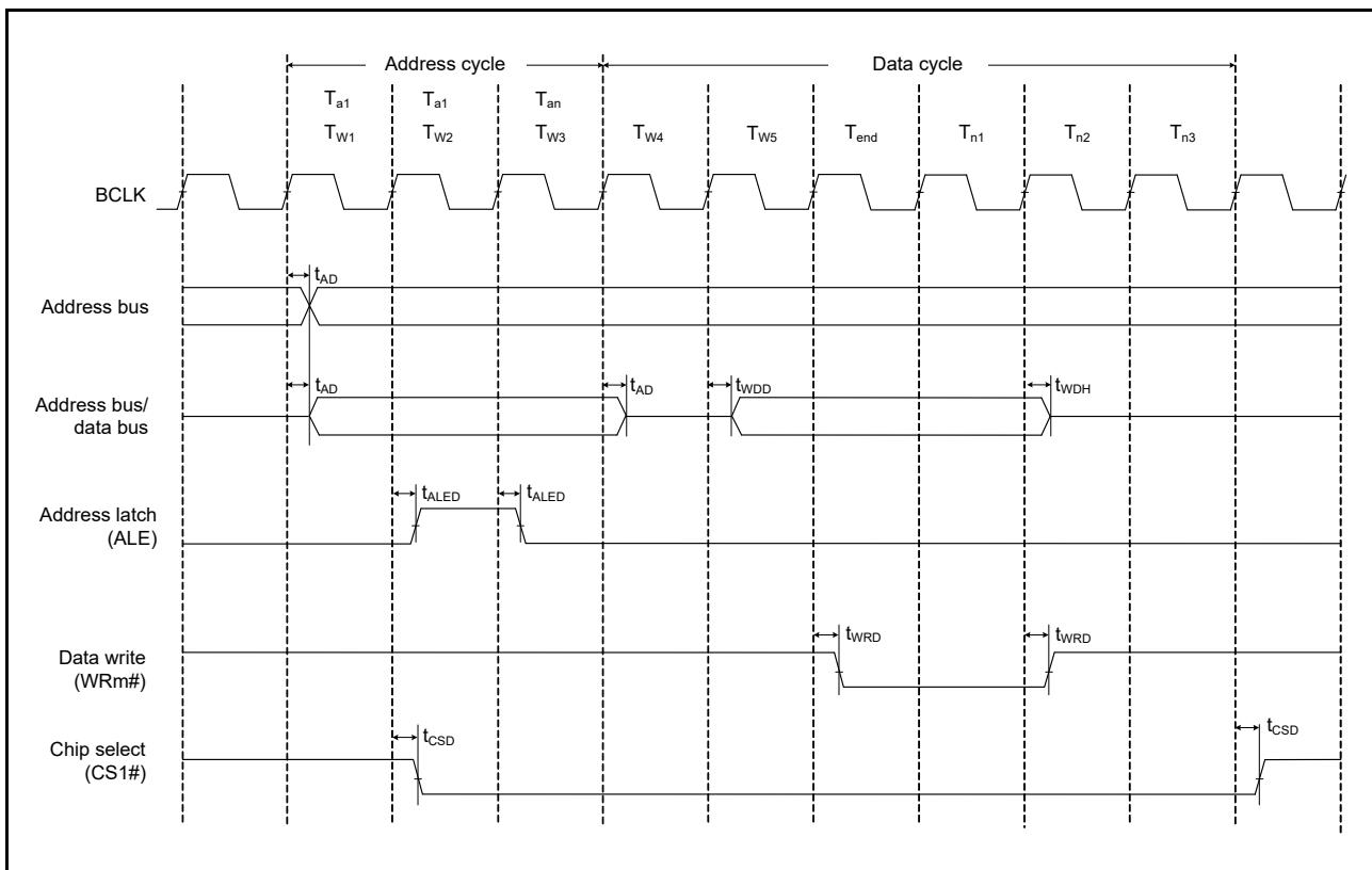
Figure 5.17 Address/Data Multiplexed Bus Write Access Timing
