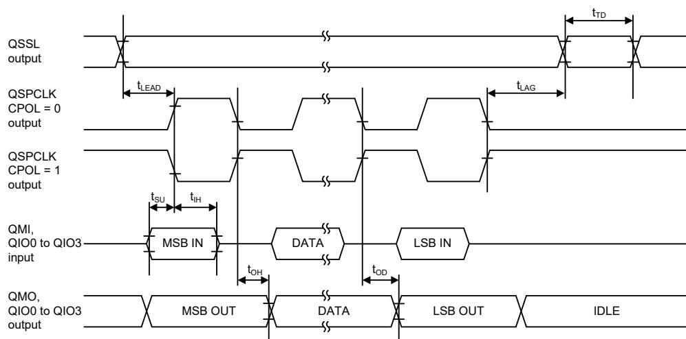
**Figure 5.54 Transmit/Receive Timing (CPHA = 0)**
