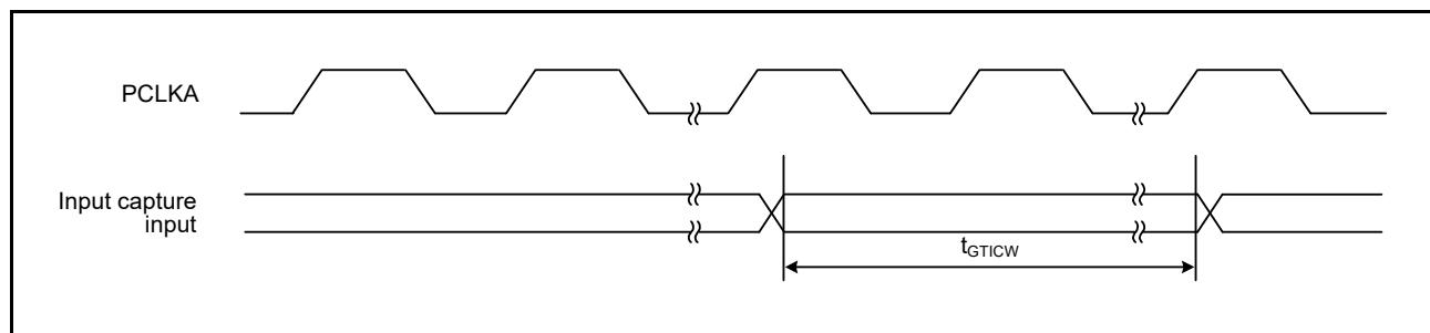
**Figure 5.41 GPT Input Capture Input Timing**
