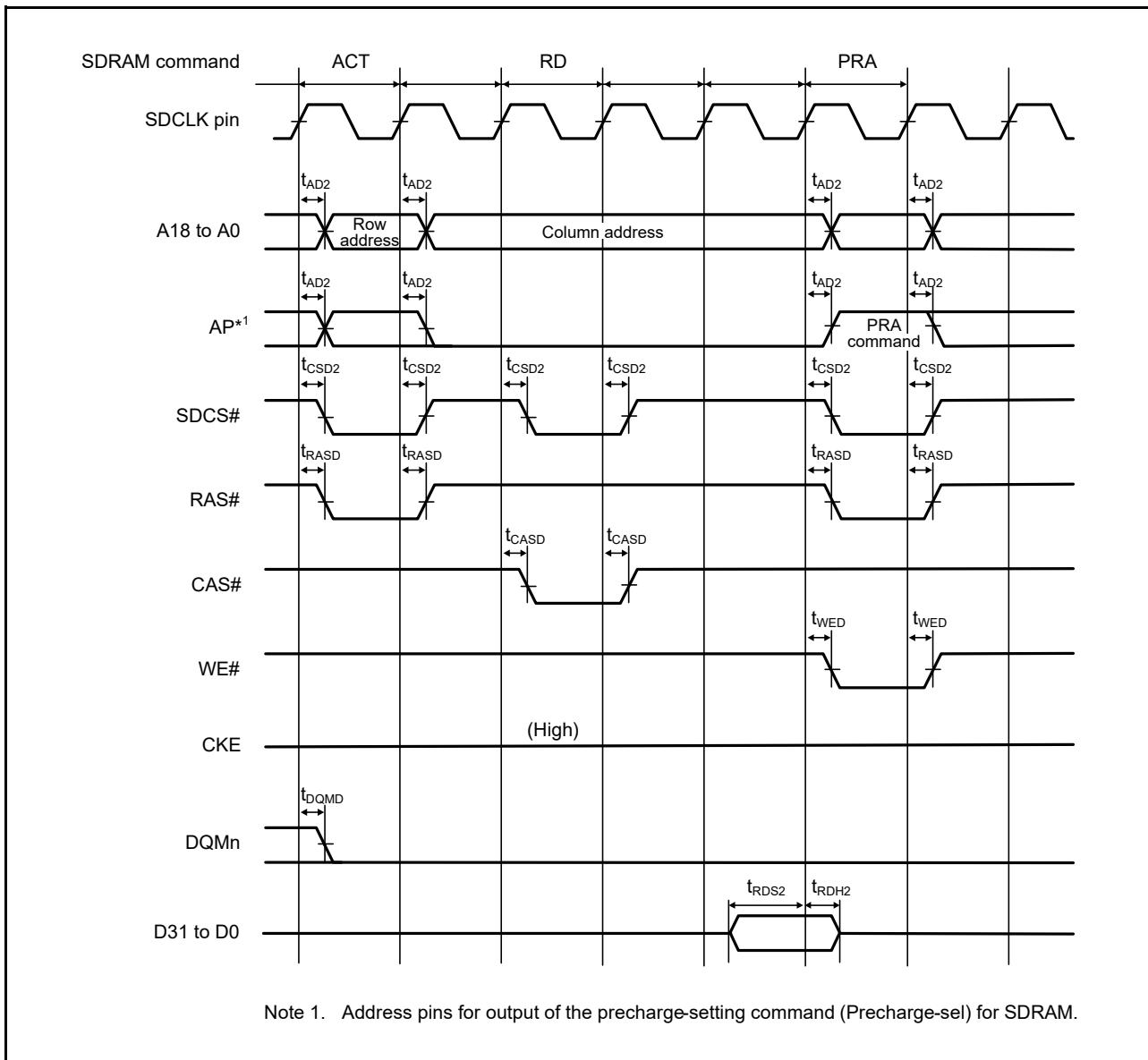
Figure 5.23 SDRAM Space Single Read Bus Timing
