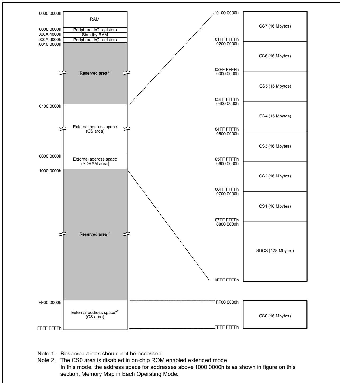
**Figure 3.2 Correspondence between External Address Spaces and CS Areas
