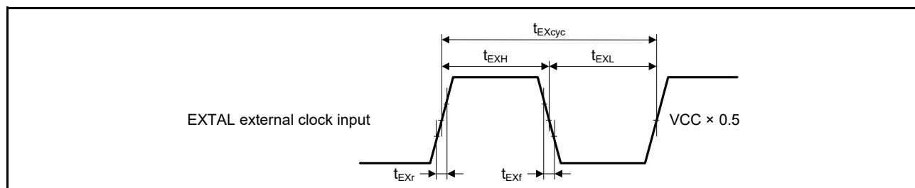
**Figure 5.4 EXTAL External Clock Input Timing****Table 5.15 Main Clock Timing**
