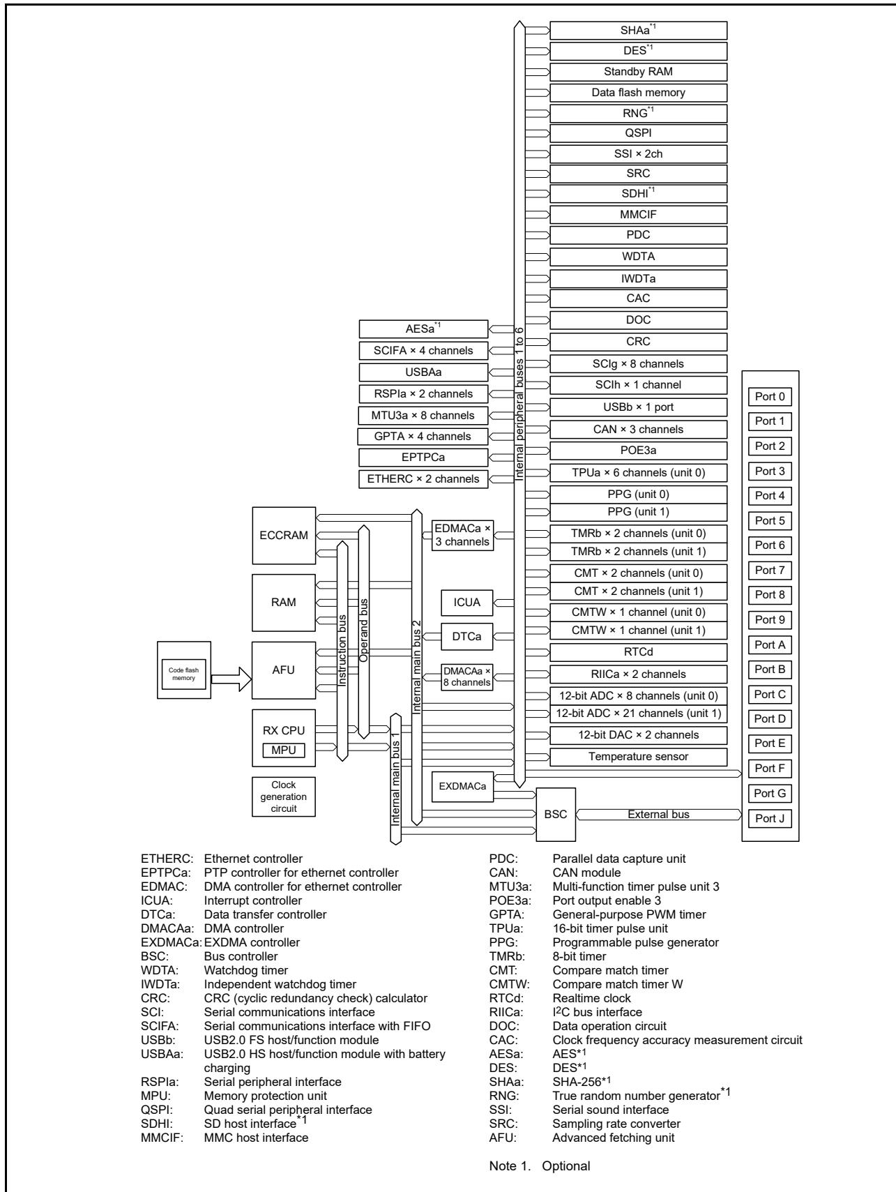
Figure 1.2 Block Diagram
