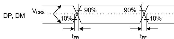
**Figure 5.77 DP and DM Output Timing (Full-Speed)**
