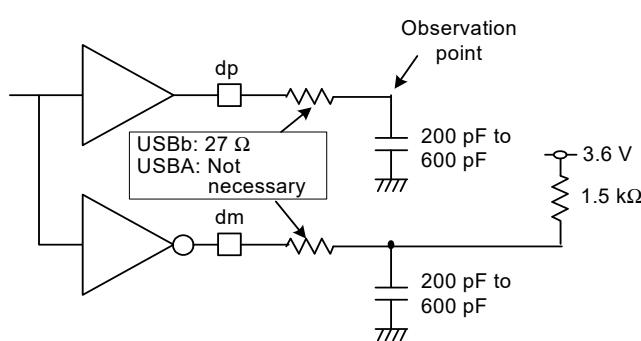
**Figure 5.76 Test Circuit (Low Speed)**
