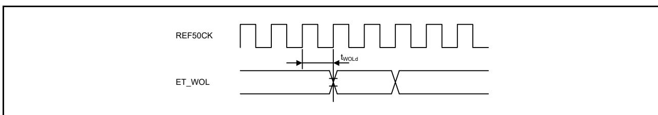
**Figure 5.66** WOL Output Timing (RMII)
