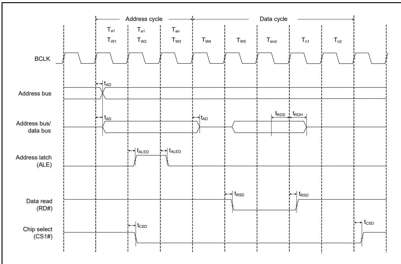
Figure 5.16 Address/Data Multiplexed Bus Read Access Timing
