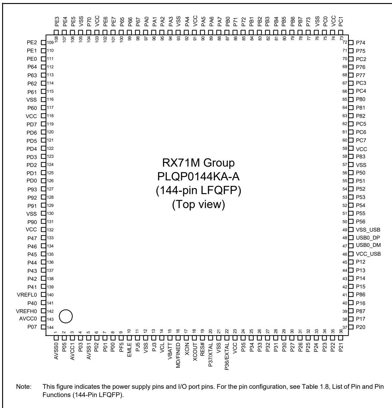
Note: This figure indicates the power supply pins and I/O port pins. For the pin configuration, see Table 1.8, List of Pin and Pin Functions (144-Pin LFQFP).
