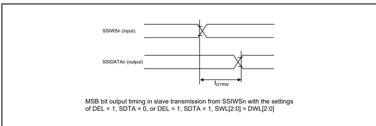
Figure 5.60 SSIDATA Output Delay from SSIWSn Change Edge
