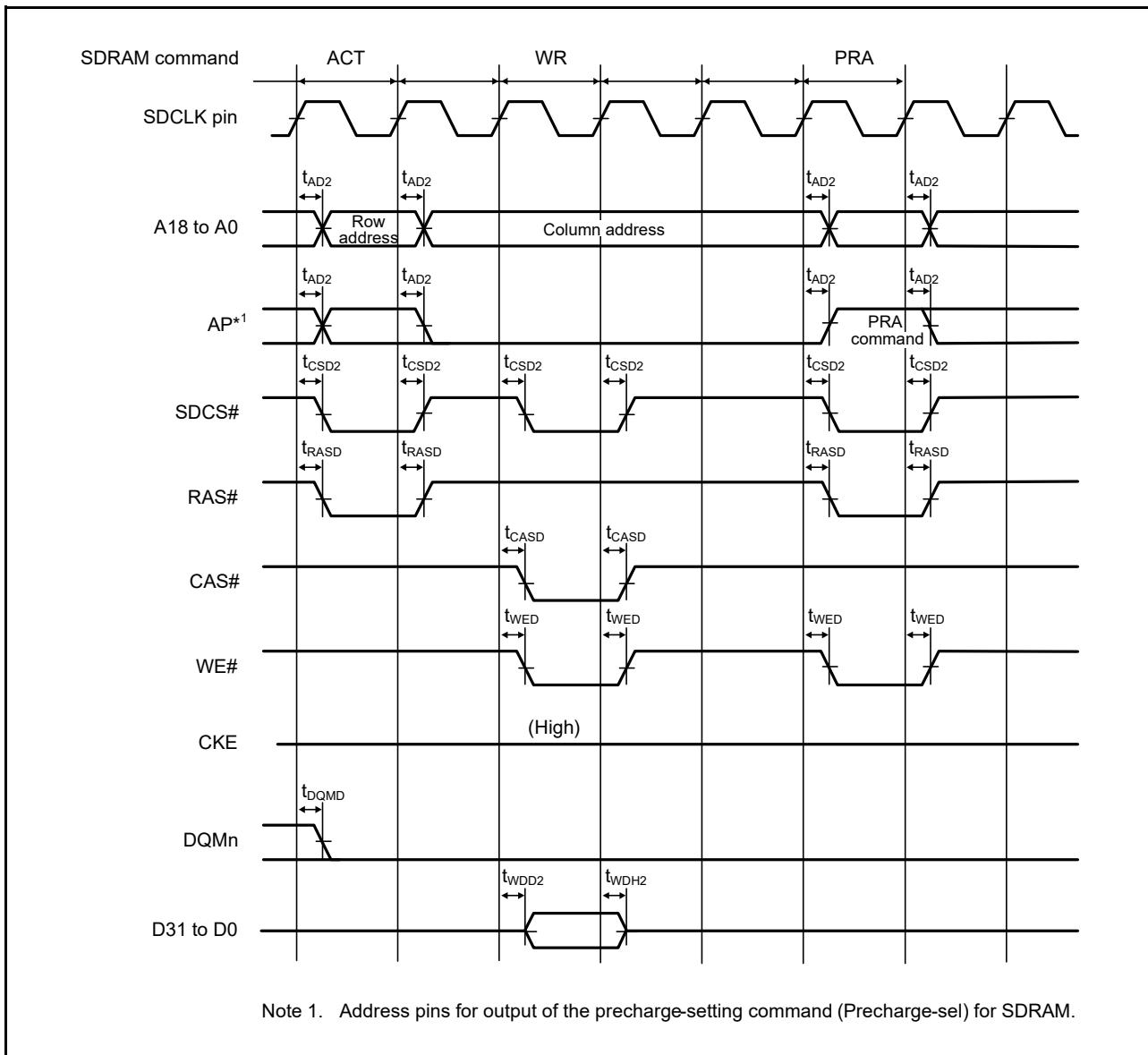
Figure 5.24 SDRAM Space Single Write Bus Timing
