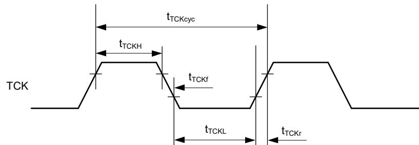
**Figure 5.90 Boundary Scan TCK Timing**
