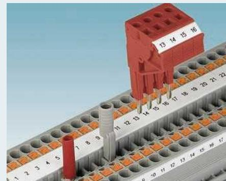
The reducing bridge allows terminal blocks with different nominal cross sections to be connected with ease. It can be used to quickly create power blocks, e.g., a 10 mm<sup>2</sup> terminal block with a 2.5 mm<sup>2</sup> or 4 mm<sup>2</sup> terminal block, regardless of the connection technology.
