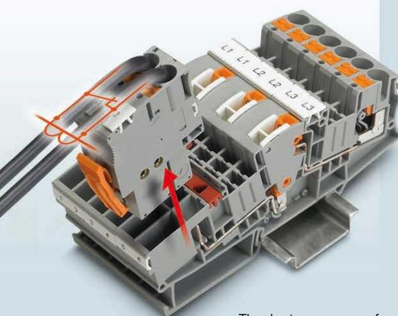
The plug-in current transformer disconnect terminal blocks also enable the safe plug-in wiring of current transformers. When the transformer plug is removed, a leading current transformer short circuit is automatically ensured. Additional coding accessories prevent the plug's polarity from being reversed.
