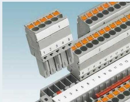
The COMBI connection system enables a plug-in wiring solution up to a nominal current of 41 A and a nominal voltage of 1000 V to be implemented. The contact system meets the most stringent of vibration requirements due to the integrated covering spring.
