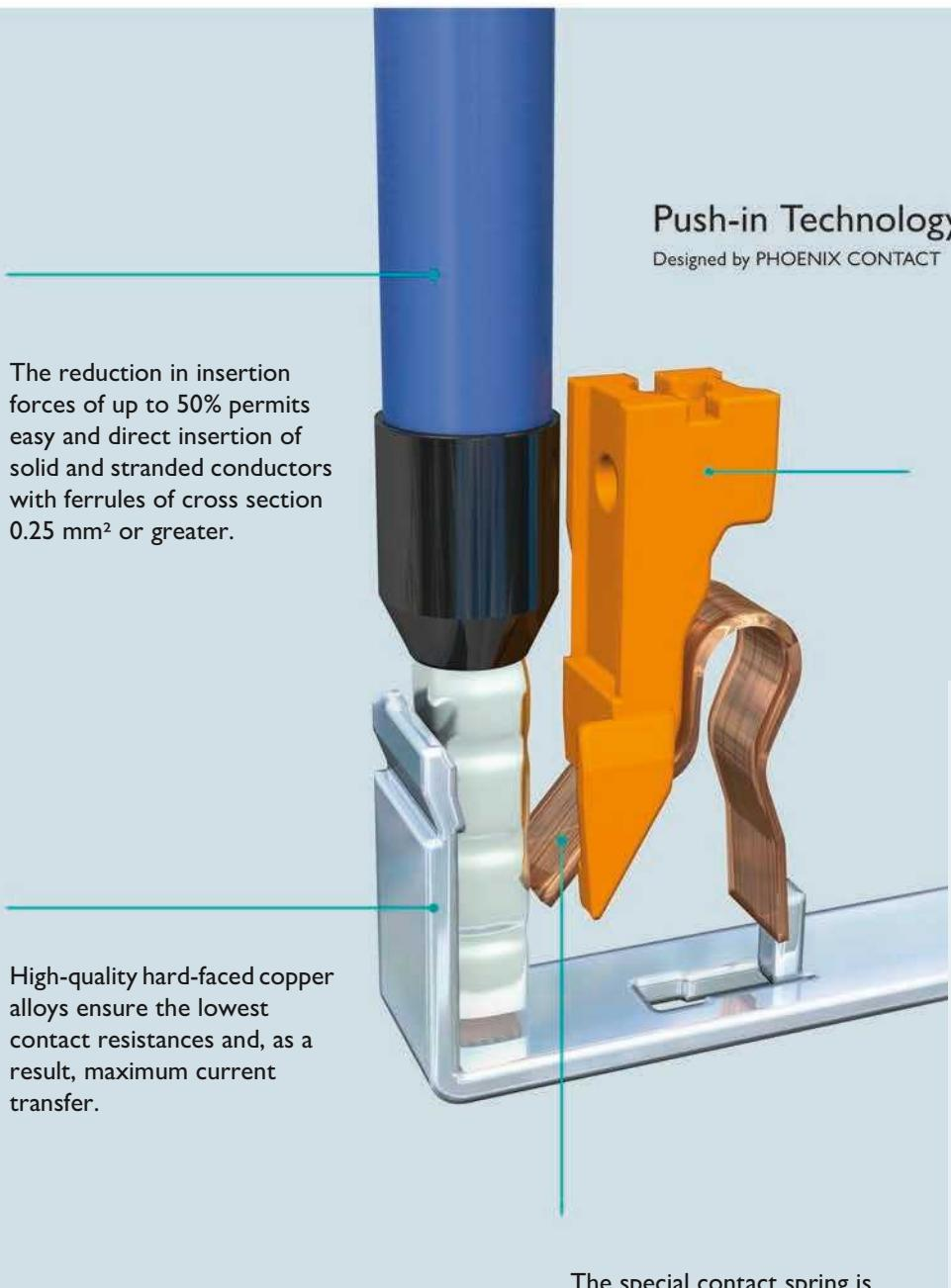
The integrated lever enables you to release connected conductors using any type of tool – easily and without direct contact with live parts. Stranded conductors of cross section 0.14 mm<sup>2</sup> and above can be connected without ferrules using the actuation lever.
