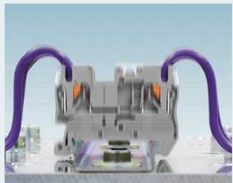
The push-in connection technology is tested for maximum vibration and shock resistance. The test runs through a frequency range of 5 Hz to 150 Hz at a speed of up to 5.72 m/s<sup>2</sup>. The test objects are tested on each of the three axes (x, y, z). No contact interruptions > 1 µs are permitted during the test. Push-in connection technology meets these high requirements in terms of vibration and shock loads up to 350 g.
