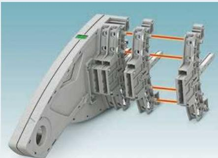
The test plug provides three function shafts. Horizontally aligned, as leading short-circuit jumper - vertically aligned as through connection in the plug. Staggered test sockets enable the use of safety test leads in a confined space.
