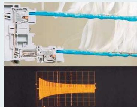
Correctly wired modular conductor contact points must offer a high degree of mechanical safety. The new push-in connection technology, requiring up to 50% lower conductor insertion forces, achieves 180 N in the conductor pull-out test of a 2.5 mm<sup>2</sup> terminal block with a 1.0 mm<sup>2</sup> conductor, for example, where only 35 N is required according to the standard.
