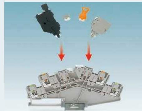
The actuation cross on the disconnect knife enables the use of different size screwdrivers. All terminal blocks offer an additional test contact on both sides of the disconnect point for test plugs with a 2.3 mm diameter.
