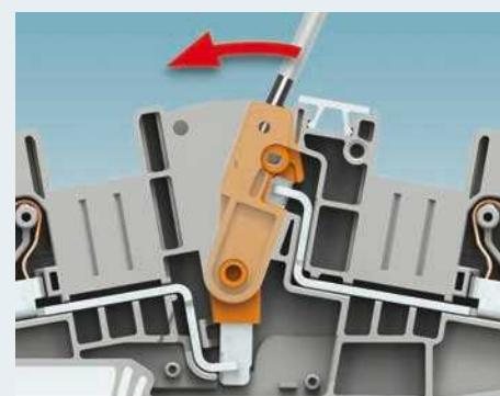
The section disconnector reliably makes contact and latches with a swiveling movement in the respective switching state. Switching symbols and optional switching locks also ensure a clear overview inside the measuring transducer terminal strip.
