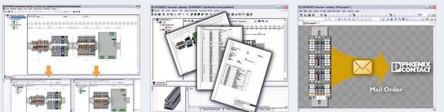
The configured terminal strips can be distributed across several DIN rails in order to determine the exact space requirements for installation.
