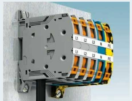
With the fully isolated and snap-on (optional) tap-off terminal block, you can easily achieve your voltage pick-off for two conductors up to 16 mm<sup>2</sup>. Large-surface marking and integrated 2.3 mm test connections.
