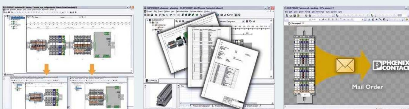
The configured terminal strips can be distributed across several DIN rails in order to determine the exact space requirements for installation.
