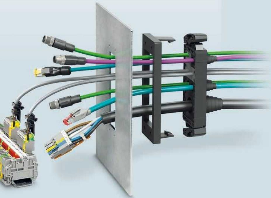
The CES cable entry system allows you to insert a variety of pre-assembled conductors, cables, and protective hoses into areas with limited space in control cabinets, distributor boxes or devices, in a way which protects them against water and dust.
