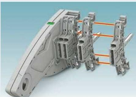
The test plug provides three function shafts. Horizontally aligned, as leading short-circuit jumper - vertically aligned as through connection in the plug. Staggered test sockets enable the use of safety test leads in a confined space.
