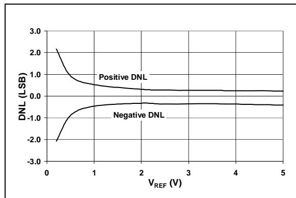
**FIGURE 2-9:** Differential Nonlinearity (DNL) vs.  $V_{REF}$ .
