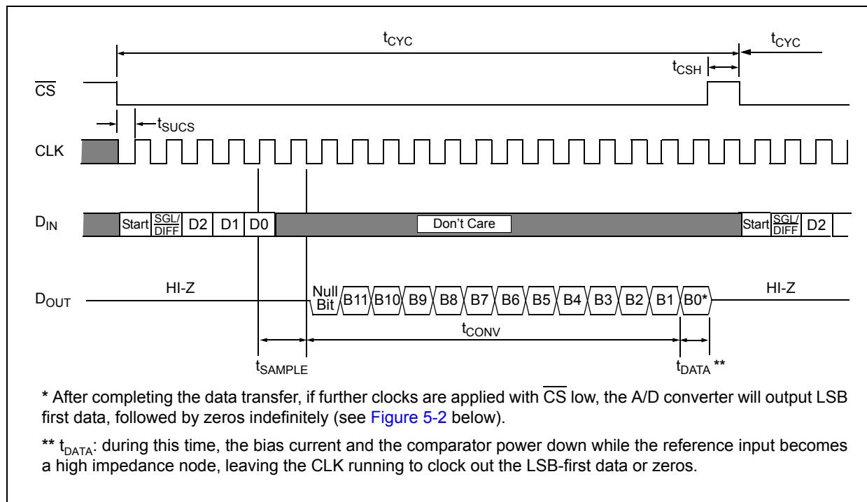
**FIGURE 5-1:** Communication with the MCP3204 or MCP3208.
