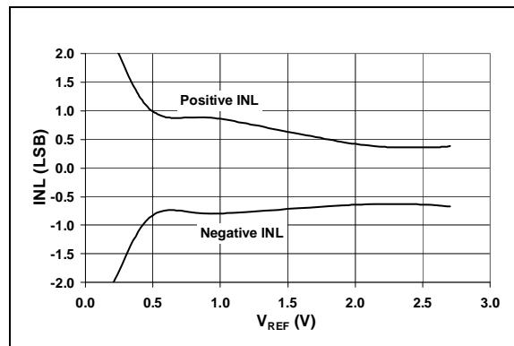
**FIGURE 2-5:** Integral Nonlinearity (INL) vs.  $V_{REF}$  ( $V_{DD} = 2.7V$ ).
