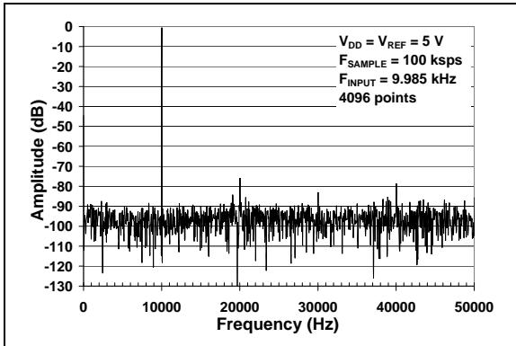
**FIGURE 2-27:** Frequency Spectrum of 10 kHz input (Representative Part).
