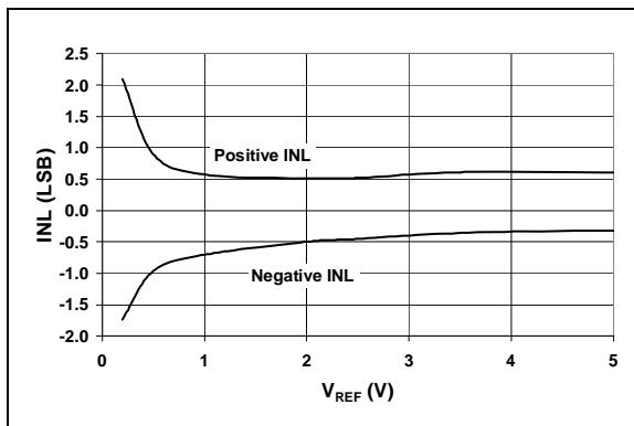
**FIGURE 2-2:** Integral Nonlinearity (INL) vs.  $V_{REF}$ .
