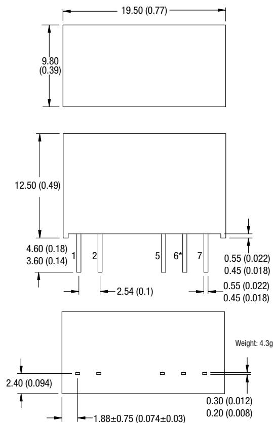
All dimensions in mm  $\pm 0.25$ mm (inches  $\pm 0.01$ ). All pins on a 2.54 (0.1) pitch and within  $\pm 0.25$  (0.01) of true position.
