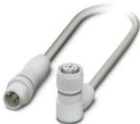
Sensor/Actuator cable, 4-position, PP-EPDM halogen-free, Gray RAL 7035, Plug straight M12, A-coded, on Socket angled M12, A-coded, Cable length: 0.6 m, Hygienic design, with plastic knurl
