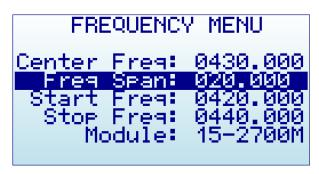
Selecting a span of 10MHz, the Start/Stop frequency changes accordingly:
