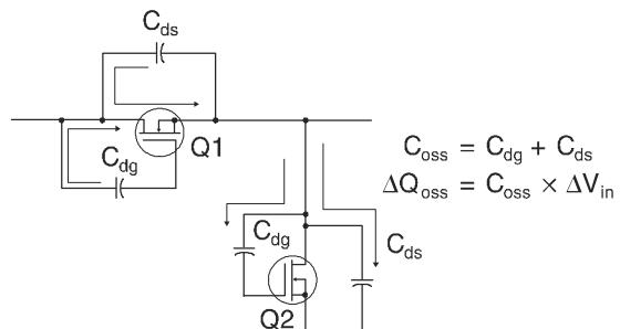
Figure 2:  $Q_{oss}$  Characteristic
