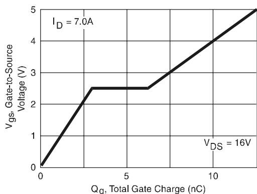
Figure 7. Typical Gate Charge vs. Gate-to-Source Voltage
