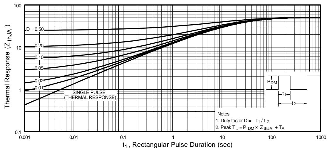
Figure 13. Maximum Effective Transient Thermal Impedance, Junction-to-Ambient
