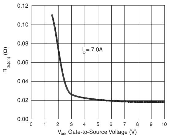
Figure 10. Typical R<sub>ds(on)</sub> vs. Gate-to-Source Voltage
