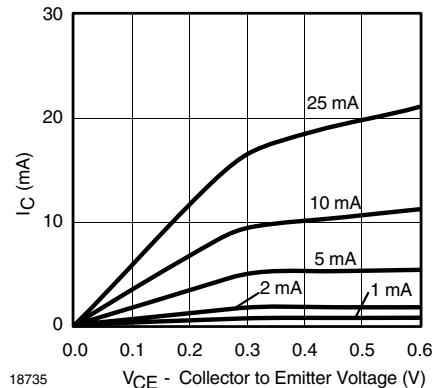
Figure 5. Normalized Current vs. Collector Emitter Saturation
