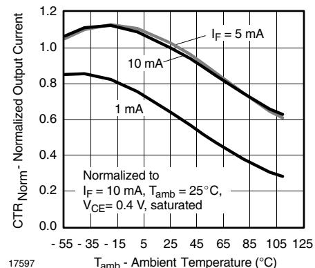
Figure 6. Normalized Current Transfer Ratio vs. Ambient
