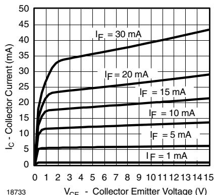
Figure 3. Collector Current vs. Collector Emitter Voltage
