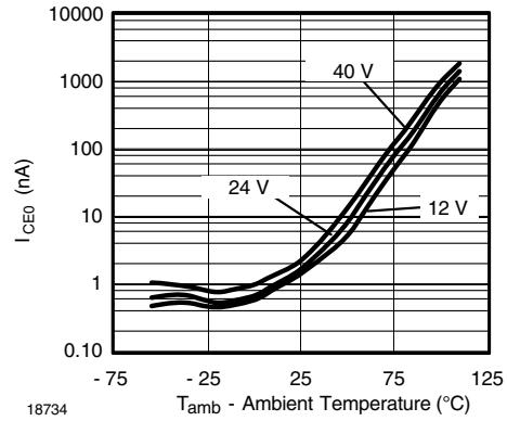
Figure 4. Collector to Emitter Dark Current vs. Ambient
