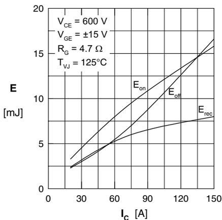
Fig. 7 Typical switching losses vs. collector current
