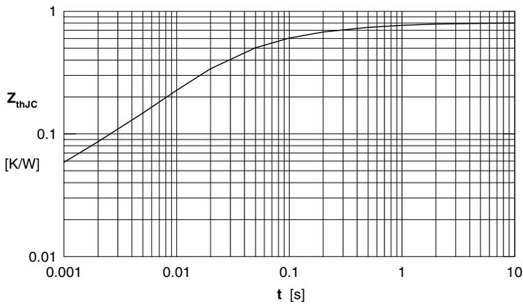
Fig. 2 Transient thermal impedance junction to case
