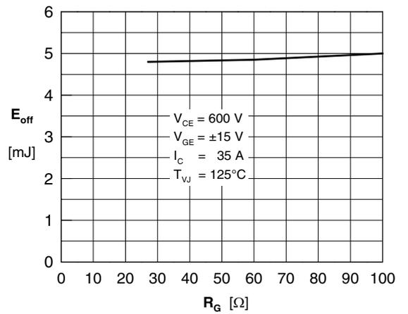
Fig. 13 Typ. turn off energy vs. gate resistor
