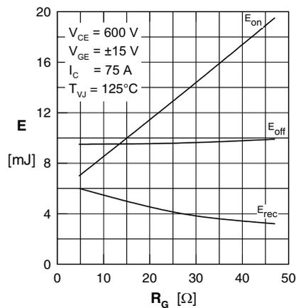
Fig. 8 Typ. switching losses vs. gate resistance
