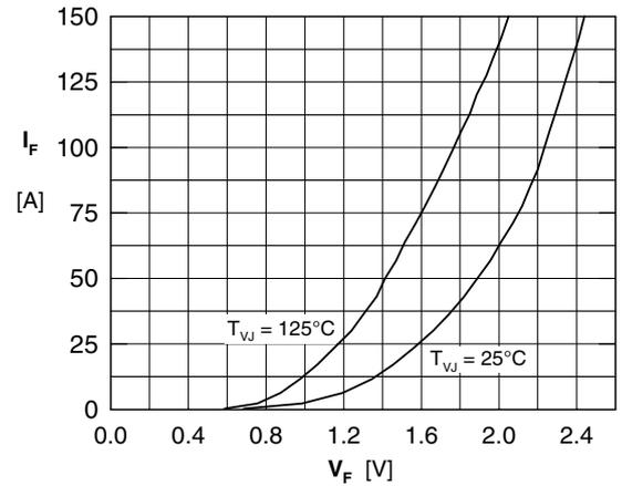
Fig. 6 Typical forward characteristic of free wheeling diode
