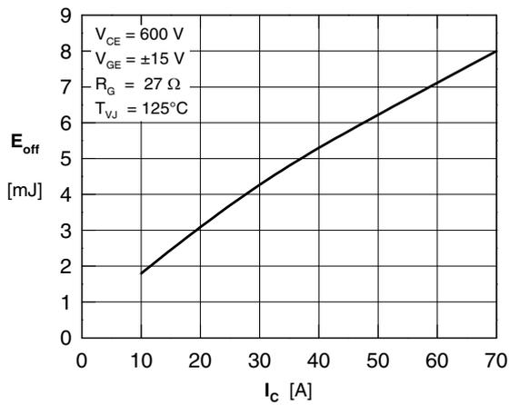
Fig. 12 Typ. turn off energy vs. collector current
