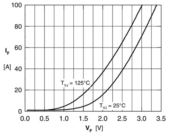
Fig. 11 Typical forward characteristics of free wheeling diode
