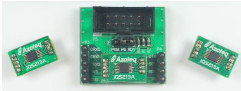
Figure 4.1 Prototype Board (center) and Module Boards (left, right and plugged into center board)
