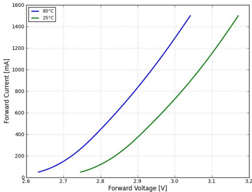
Figure 4a. Typical forward current vs. forward voltage for LUXEON F Plus Cool White at  $T_c=85^\circ\text{C}$ .
