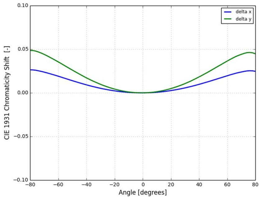
Figure 5b. Typical color shift in CIE 1931 x, y coordinates over angle for LUXEON F Plus Cool White at 20ms MP, 1000mA.
