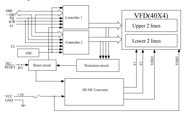
Upper 2 lines are controlled by Controller 1 with E1 signal, and Lower 2 lines are controlled by Controller 2 with E2 signal.
