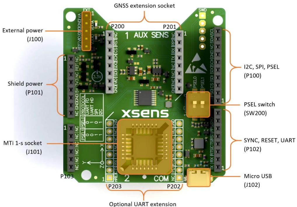
Figure 7: MTi 1-series Shield Board with connector designators
