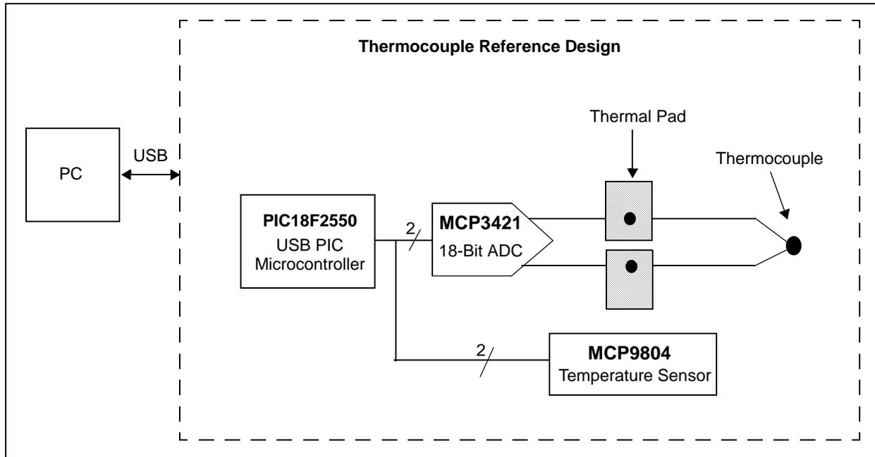
**FIGURE 2-1:** *Thermocouple Reference Design Simplified Block Diagram.*
