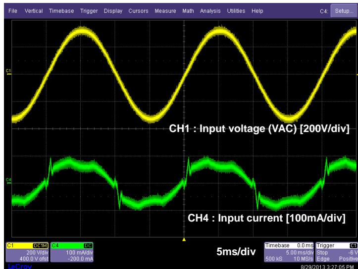
Figure6. Input waveform
