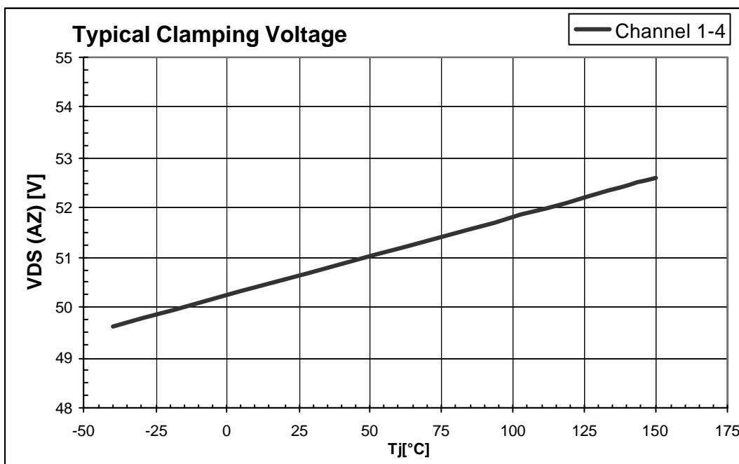
**Figure 7 :** Typical Clamp Voltage versus Junction-Temperature
