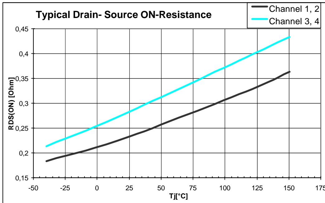
**Figure 6 :** Typical ON Resistance versus Junction-Temperature
