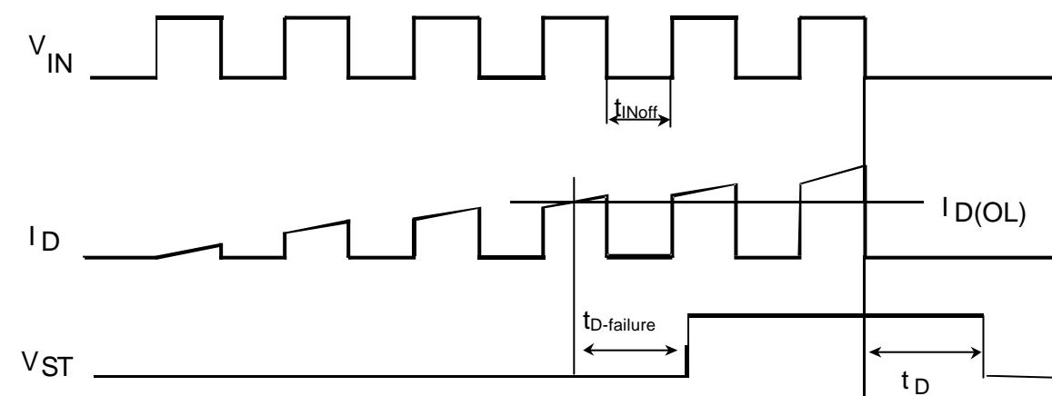
$t_{INoff} < t_D$  leads to a static status signal
