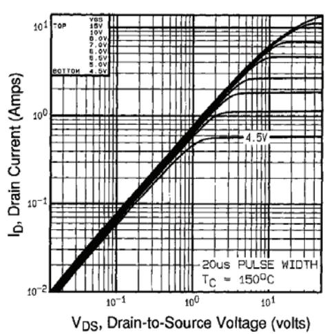
Fig. 2 - Typical Output Characteristics,  $T_C = 150^\circ\text{C}$
