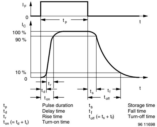
Fig. 2 - Switching Times
