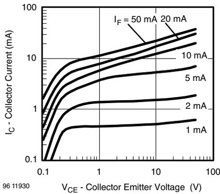
Fig. 8 - Collector Current vs. Collector Emitter Voltage
