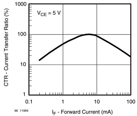
Fig. 10 - Current Transfer Ratio vs. Forward Current
