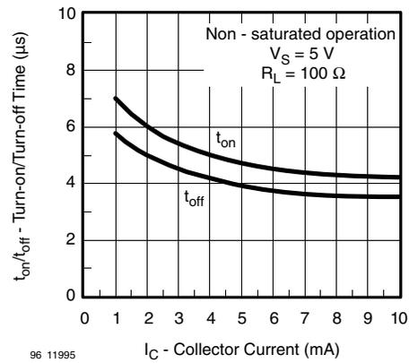
Fig. 11 - Turn-on/Turn-off Time vs. Collector Current
