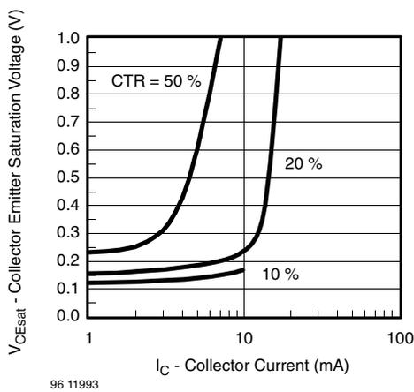
Fig. 9 - Collector Emitter Saturation Voltage vs. Collector Current
