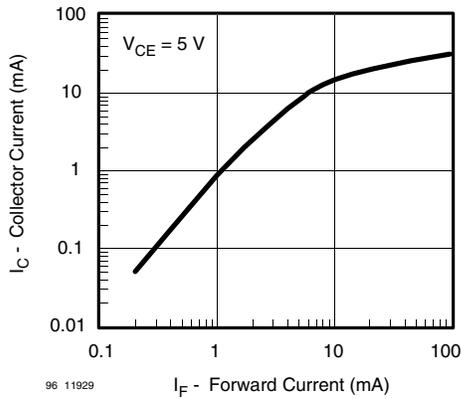
Fig. 7 - Collector Current vs. Forward Current
