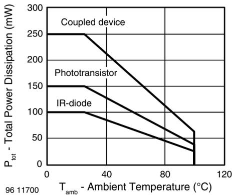
Fig. 3 - Total Power Dissipation vs. Ambient Temperature
