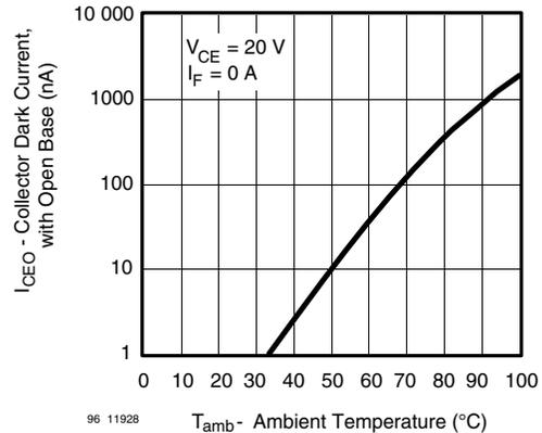
Fig. 6 - Collector Dark Current vs. Ambient Temperature
