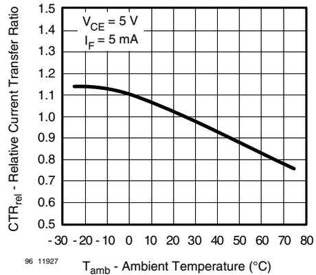
Fig. 5 - Relative Current Transfer Ratio vs. Ambient Temperature
