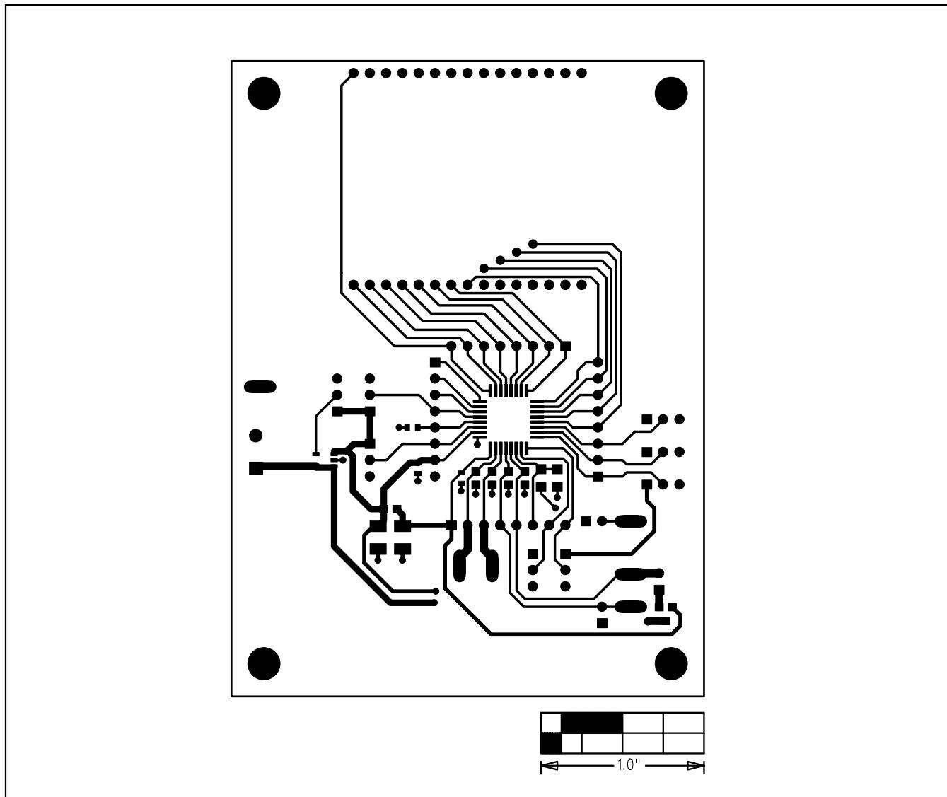
Figure 3. MAX1493 EV Kit PCB Layout—Component Side
