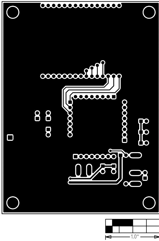
Figure 4. MAX1493 EV Kit PCB Layout—Solder Side
