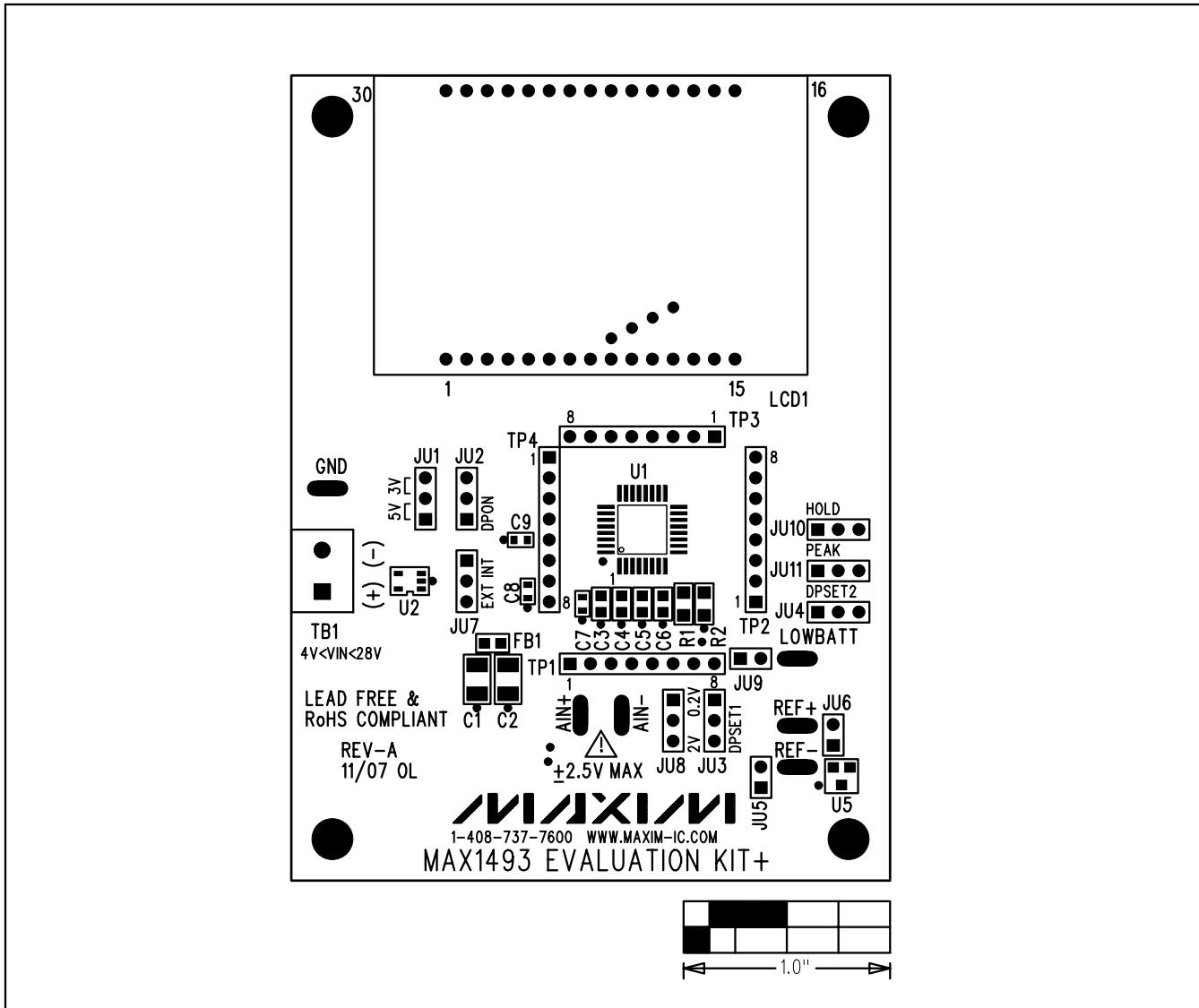
Figure 2. MAX1493 EV Kit Component Placement Guide—Component Side
