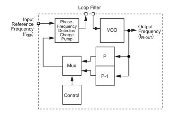
Figure 1. Fractional-N Synthesizer Architecture
