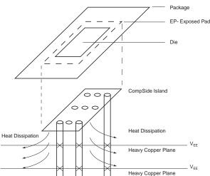
PCB Thermal Consideration for 32-Pin EPAD-TQFP Package
