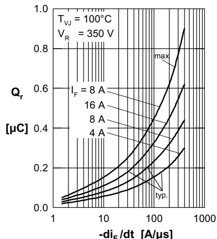
Fig. 2 Typ. reverse recov. charge
