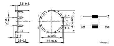
Tolerances to ISO 2768-C unless otherwise noted. Dimensions in mm.
