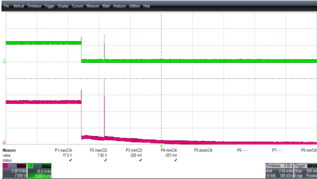
Figure 42 – Output Voltage Waveform. 85 VAC Input. Upper: 12 V, 10 V / div. Lower: 5 V, 2 V / , 2 s / div.
