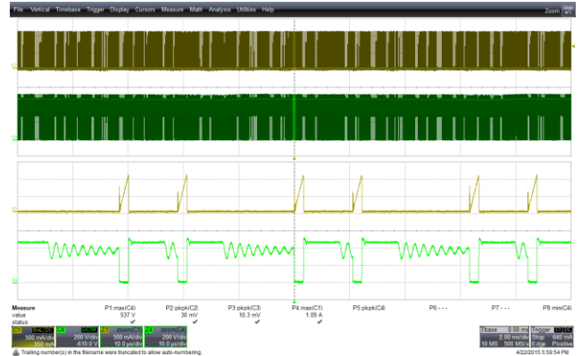
Figure 31 – Drain Voltage and Current Waveforms. 265 VAC Input, Full Load, (537 V_{MAX} ). Lower: I_{DRAIN} , 500 mA / div. Upper: V_{DRAIN} , 200 V, 2 ms, 10 \mu s / div.
